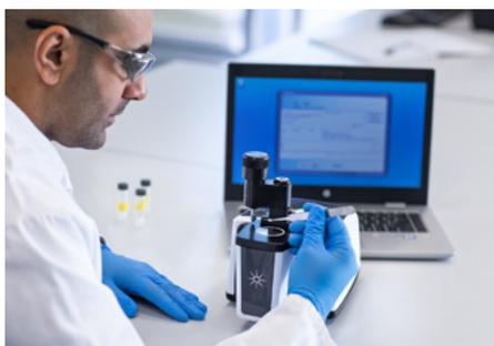
The Agilent Cary 630 FTIR spectrometer is a flexible benchtop FTIR spectrometer that offers high-performance and extraordinary ease of use for cutting-edge research and routine analysis alike. When equipped with the ATR accessory, it enables fast identification of larger microparticles in the size range from around 300µm up to 5mm.
