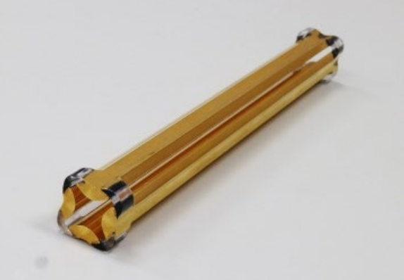
Gold plated fused silica quad from 5973 MSD
