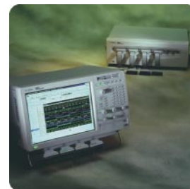
The Agilent 1680 and 1690 series logic analyzers make it easy for digital designers to examine relationships of time or data on an integrated circuit.
