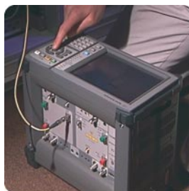
Agilent's 40 Gb/s Parallel Bit Error Ratio Test (ParBERT) platform enables R&D engineers to simulate and analyze real-world conditions of very high data rates for next-generation communication transmission lines.
