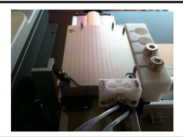
• Three fast rotary valves (six-port)
