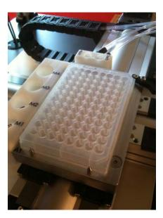
${\bf a}$   $\,$  Manually adjust the stage to clear the plate and wash station by about 0.5  $\,$  cm.
