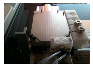
**3** With the vacuum on, check that fluid is being aspirated from the drain (central trough). Be sure not to overflow the wash station.
