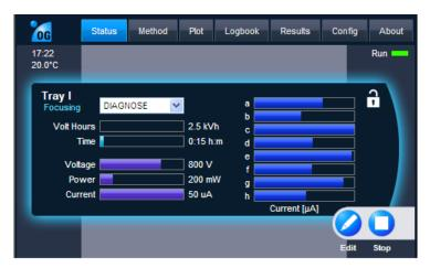
Figure 44 Typical current pattern on tray I when every lane is filled with water.
