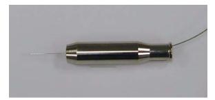
Figure 2 Needle Assembly with needle and transfer-line (or column).
