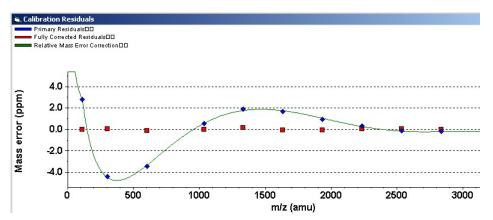
Figure 11 Detailed residual plot from negative ion calibration
