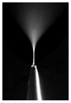
Figure 16 Nanoelectrospray plume as seen through microscope
