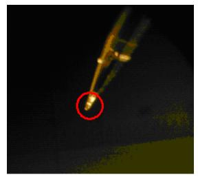
Figure 39 30 μm C18 particles aggregated just upstream of the needle tip opening. This photo actually shows too much C18 material, which is the result of dipping the needle into the suspension for 5 seconds. Only a barely discernible amount to is needed to prevent clogging.
