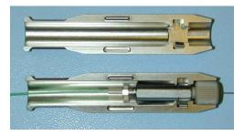
Figure 31 The needle/union/transfer assembly seated into the union holder.
