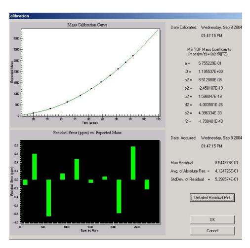
Figure 7 Calibration results (positive ion mode)
