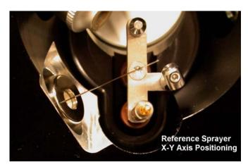
Figure 18 Reference sprayer X-Y axis positioning
