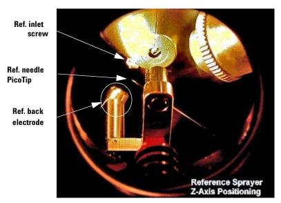
Figure 17 Reference sprayer Z-axis positioning
