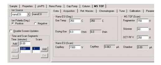
Figure 15 Example of nanoESI source parameters for LC analysis
