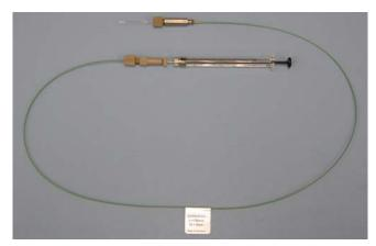
Figure 32 Completed infusion assembly with union holder (clamshell) removed for clarity.
