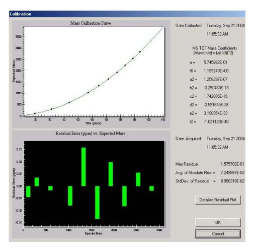
Figure 10 Calibration results (negative ion mode)
