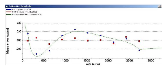
Figure 8 Detailed residual plot from positive ion calibration
