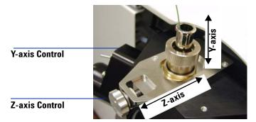
Figure 12 Adjustment of the needle position in the vertical direction uses the Y-axis control knob. Adjustment of the horizontal direction, between the back electrode and inlet capillary, uses the Z-axis control knob.
