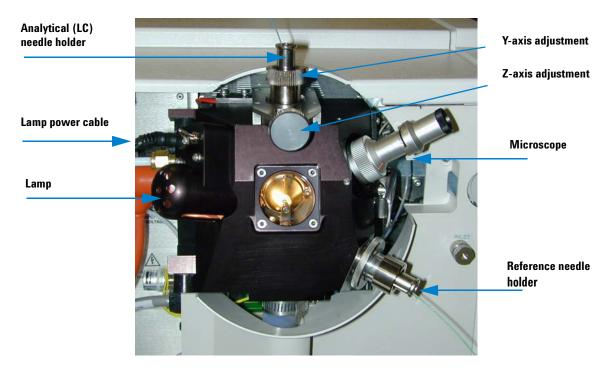
Figure 1 Dual nanospray ion source.
