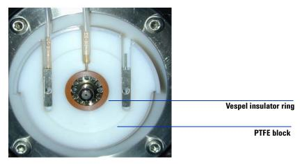
Figure 42 Spray shield, capillary cap, and endplate removed.
