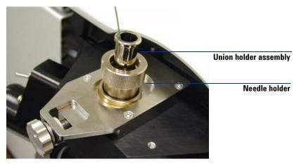
Figure 34 The union holder assembly inserted into the needle holder.
