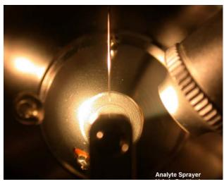
Figure 13 Needle positioned for LC analysis (front window view). Position the needle tip at the score mark between the dual-cone assembly and the back electrode.
