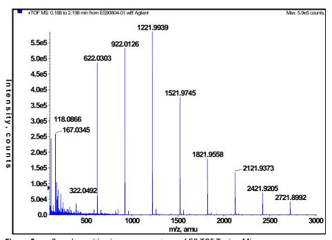
Figure 6 Sample positive ion mass spectrum of ES-TOF Tuning Mix
