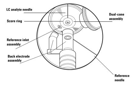
Figure 44 DNS assemblies and needle positions
