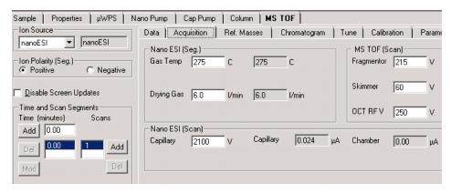
Figure 4 DNS TOF source parameters for calibration and tuning
