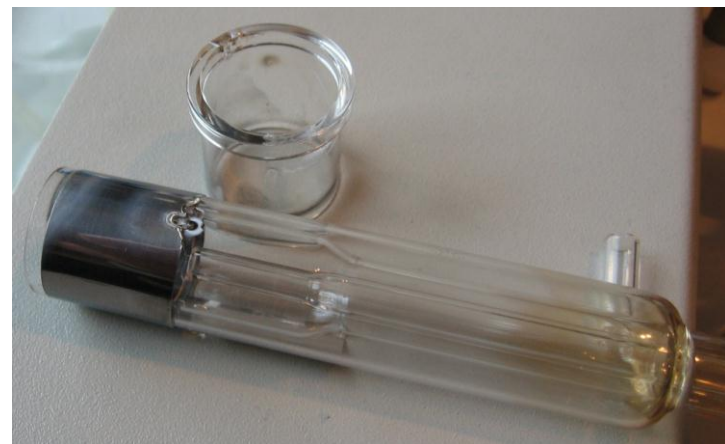
Torch damage due to incomplete drying
