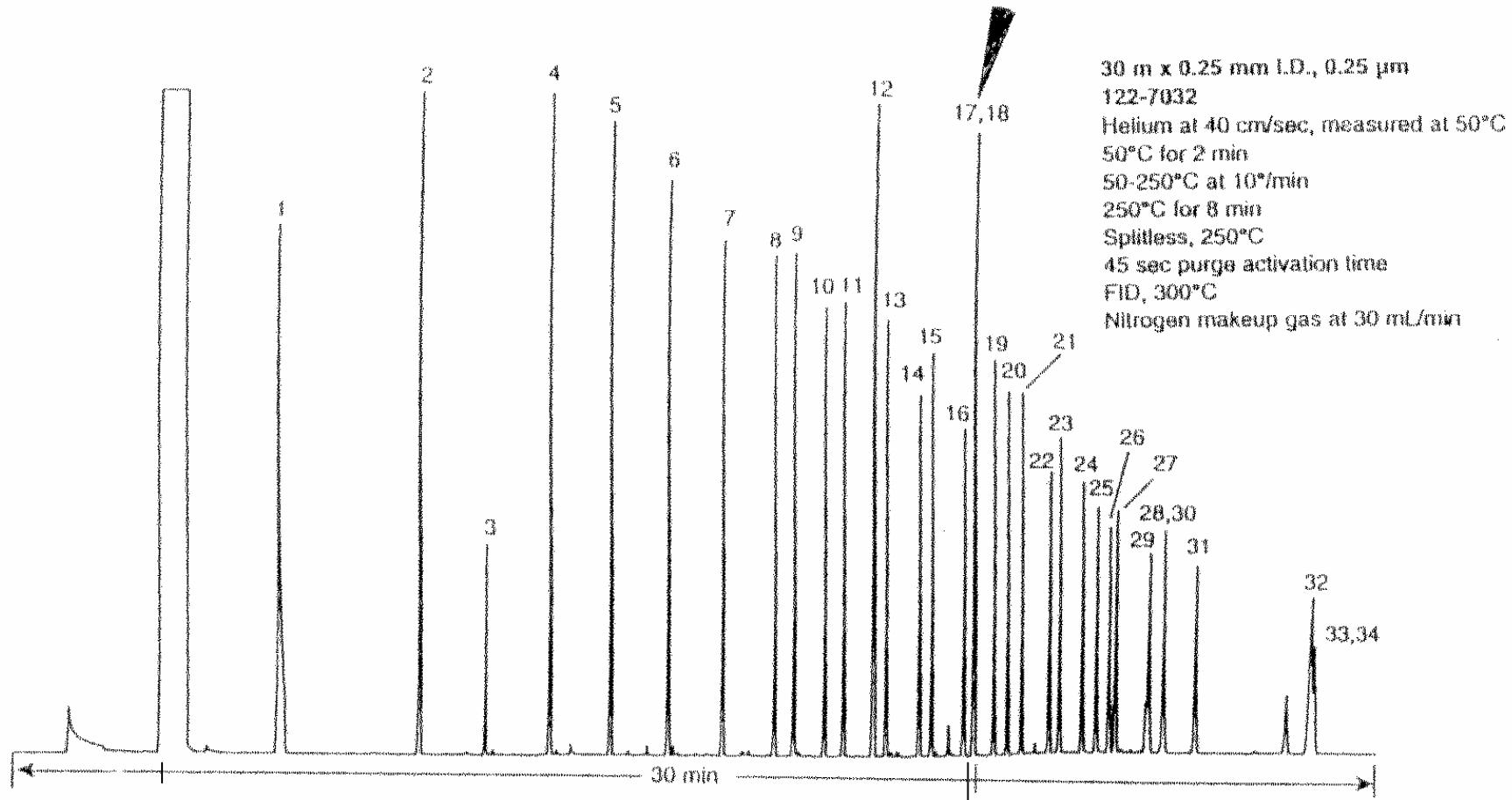
**Critical area elutes at 242°C; at 212°C, that chromatographing plug is ca. half way through the column. Set oven temperature at 212, and optimize carrier for a solute  $k = 7$ . Cool oven to 50°C starting temperature, and institute run.**
