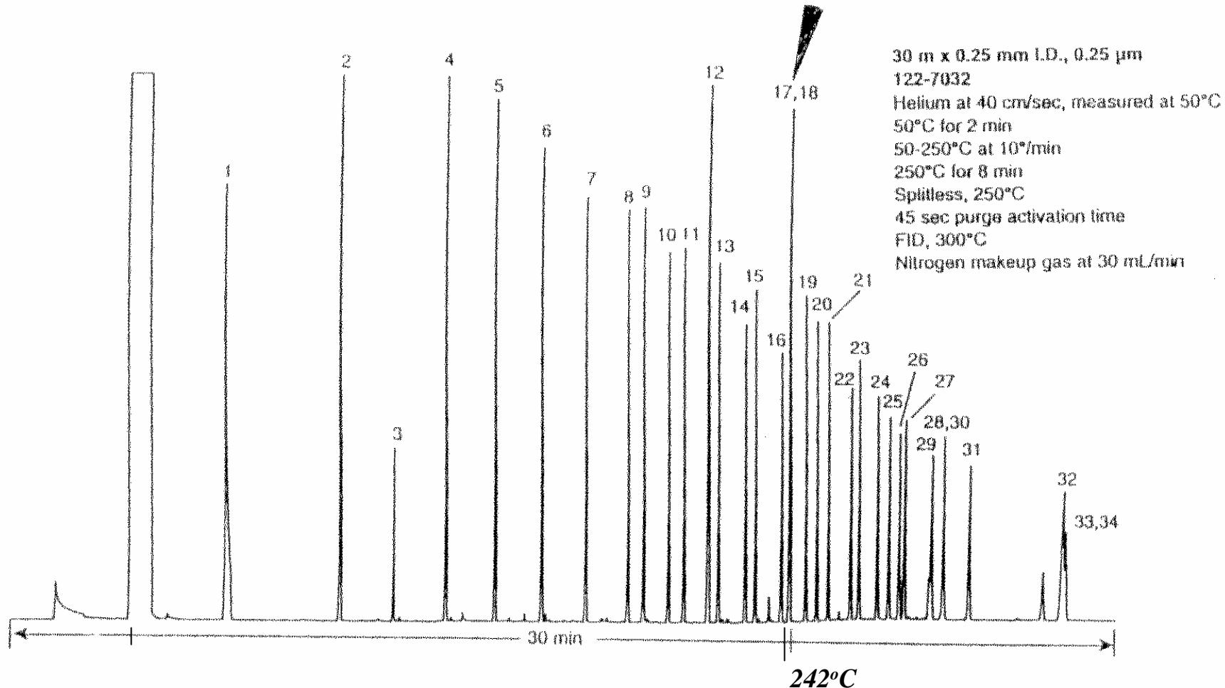
**Critical area elutes at 242°C; at 212°C, that chromatographing plug is ca. half way through the column. Set oven temperature at 212, and optimize carrier for a solute  $k = 7$ . Cool oven to 50°C starting temperature, and institute run.**
