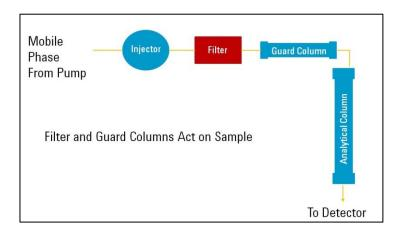
A blockage can occur in any spot, from the pump to the detector outlet. Your system should be plumbed to prevent particulates from getting to your column inlet.
