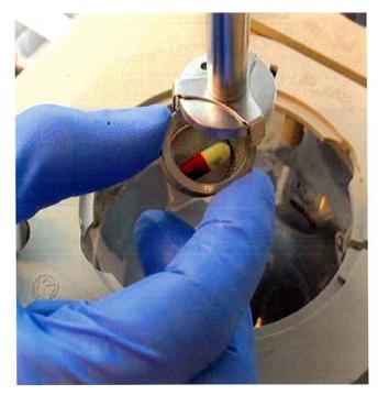
Figure 3. Placing the basket on the shaft.
