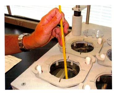
Figure 2. Temperature measurement.
