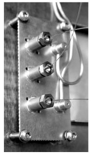
Figure 1. A close-up view of the new micro-fluidic Deans switch in the 6890N GC.
