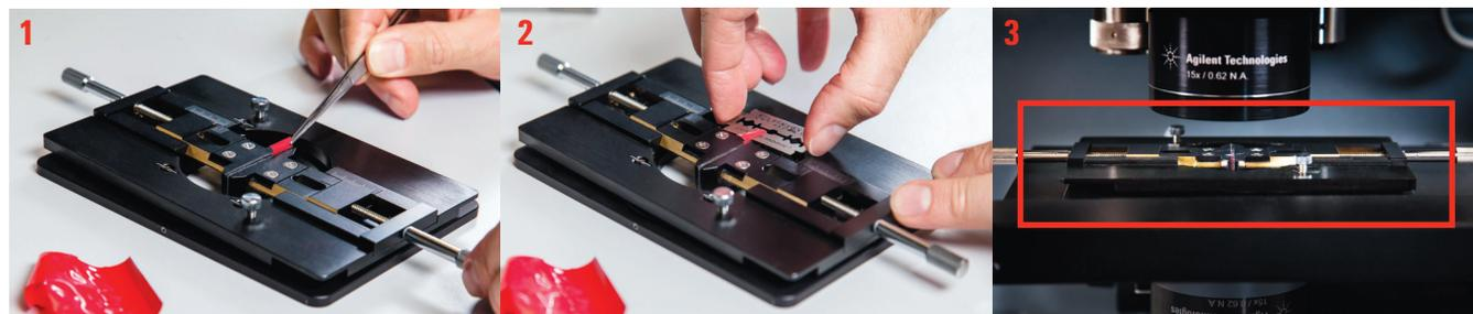
**Figure 2.** Sample mounting and analytical procedure. 1) Hold the sample in a micro-vice, 2) Cross-section the sample with a razor blade and 3) Place on microscope stage (red box), engage the ATR, and then determine answers in seconds.
