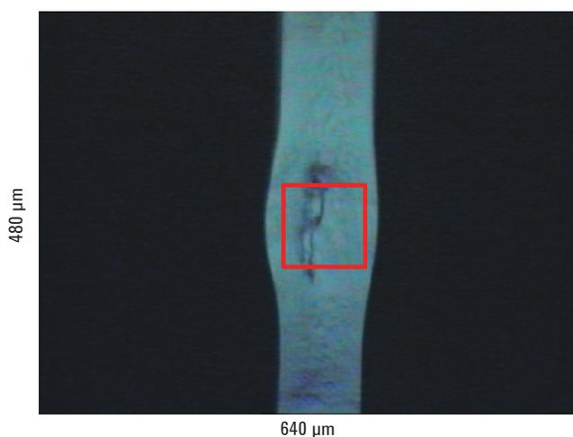
**Figure 1.** Visible image of the polymer cross-section with the defect of interest clearly visible in the center. The red box shows the location and area of the micro-ATR analysis.
