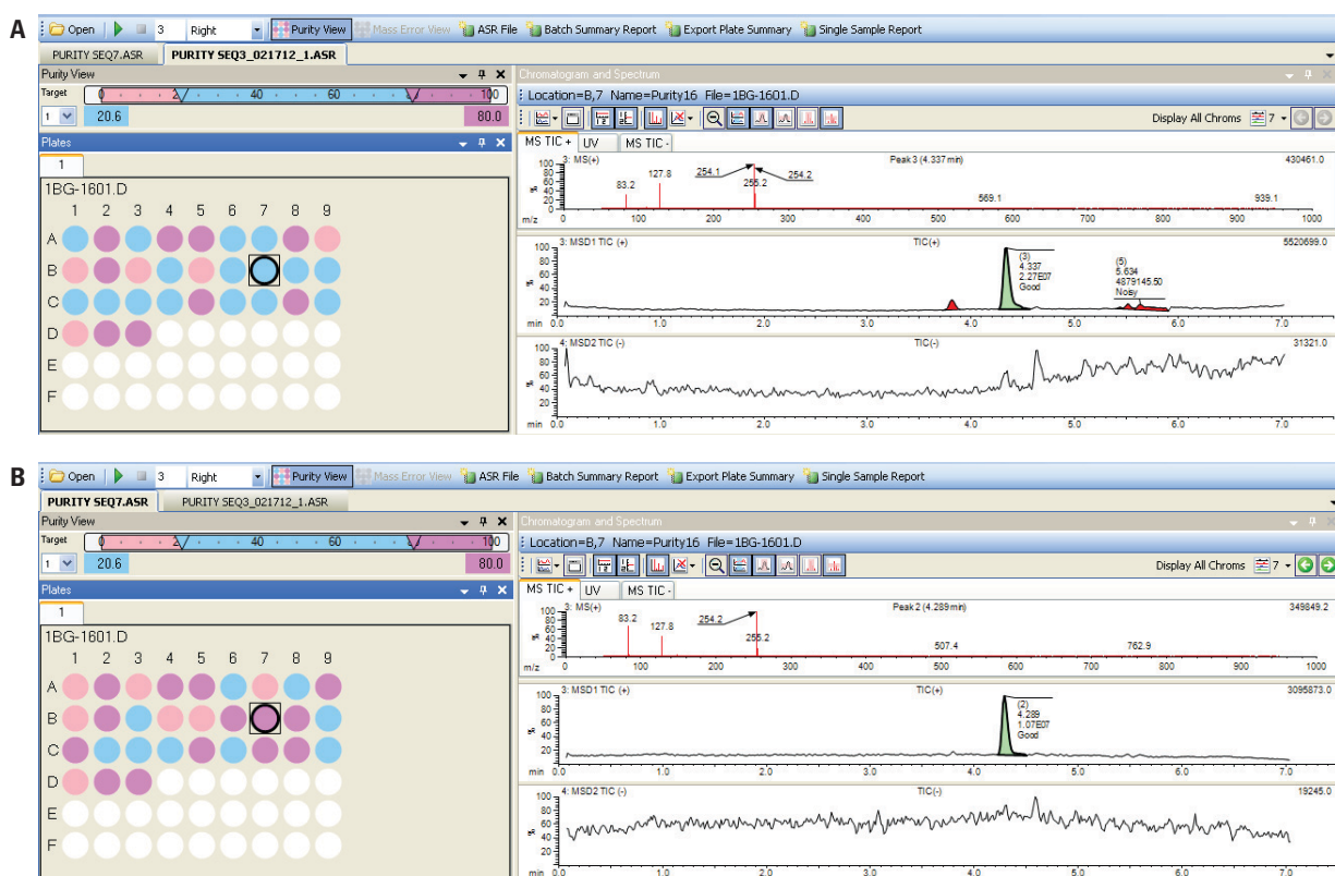
Figure 4. The comparison of purity view of the same compound library analyzed using the AJS source (A) and the ESI source (B).
