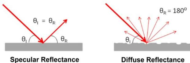
Figure 1. Specular reflectance versus diffuse reflectance
