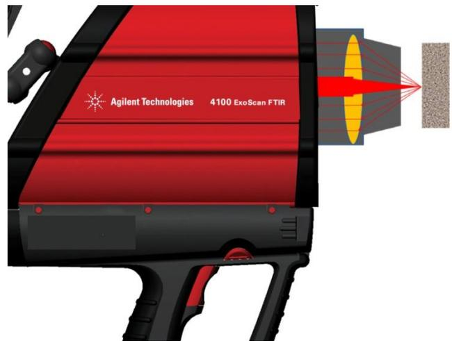
Figure 2. The diffuse reflectance sample interface provides a large collection angle to effectively collect diffusely scattered light. Additionally, the slow focus provides a large depth of field, enabling data collection even when the sample is several millimeters from the beam focus. The combination of these two features enables easy measurement on real samples, which are not always flat or smooth.
