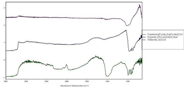
**Figure 3.** IR spectra of franklinite, esperite and willemite minerals collected on the 4100 ExoScan FTIR with diffuse reflectance
