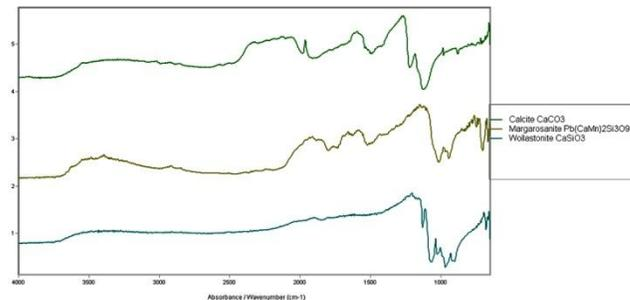
**Figure 4.** IR spectra of calcite, margarosanite and wollastonite minerals collected on the 4100 ExoScan FTIR with diffuse reflectance
