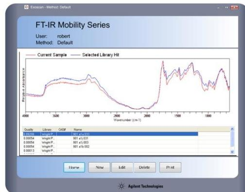
Figure 5. Library match showing identification of a polymer coating on finished product
