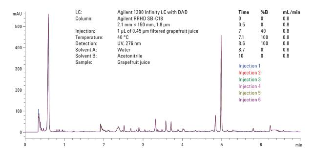
Figure 4. Overlay of six analyses with no variability in retention, selectivity or resolution, indicating sufficient column flushing and re-equilibration.
