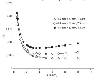
Figure 2 Plots of plate height versus velocity. Plate heights for sub-2-µm columns remain relatively constant compared to larger particle sized columns as mobile phase velocity (flow rate) increases.
