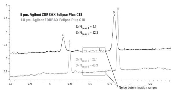
Figure 8. Signal-to-noise comparison of 5 and 1.8 µm Agilent ZORBAX Eclipse Plus C18 columns, 2.1 mm × 150 mm using a 1 ppm each quercetin and naringenin standard. Chromatographic conditions are listed in the experimental section.
