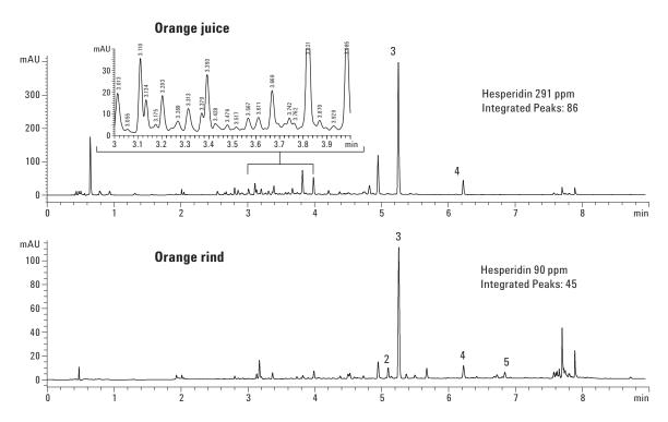
Figure 5. UHPLC fingerprint of orange juice and rind analyzed by an Agilent ZORBAX RRHD Eclipse Plus C18, 2.1 mm × 150 mm (p/n 959759-902). Chromatographic conditions are listed in experimental section.
