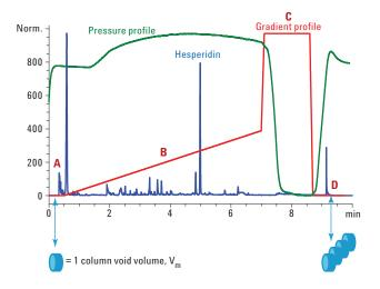
Figure 3. UHPLC of grapefruit juice with pressure and gradient profiles, and column volumes needed for re-equilibration. Segments of the gradient include A: initial isocratic hold, B: linear elution ramp, C: strong solvent column flush, D: re-equilibration.
