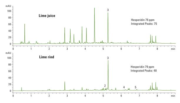
Figure 7. UHPLC fingerprint of lime juice and rind analyzed by an Agilent ZORBAX RRHD Eclipse Plus C18, 2.1 mm × 150 mm (p/n 959759-902). Chromatographic conditions are listed in experimental section.
