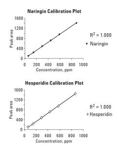
Figure 1. Chromatogram of the flavonoid standard mixture and calibration curves for naringin and hesperidin. Chromatographic conditions are listed in experimental section.
