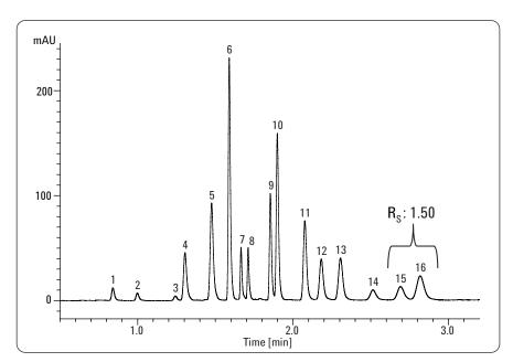
Figure 1 Separation of PAH (EPA 16) mixture on Eclipse PAH 2.1 x 50 mm, 1.8  $\mu$ m column. Critical resolution ( $R_S$ ) calculated by tangent method. Pressure limit for the column: 600 bar. Please note that a solvent blank run was subtracted.
