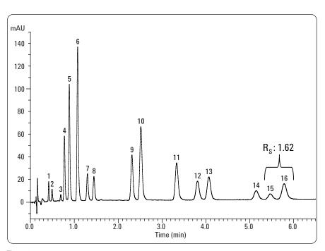
Figure 2 Separation of PAH (EPA 16) mixture on Eclipse PAH 2.1 x 50 mm, 1.8  $\mu$ m column. Critical resolution (R<sub>S</sub>) calculated by tangent method. Pressure limit for the column: 600 bar.
