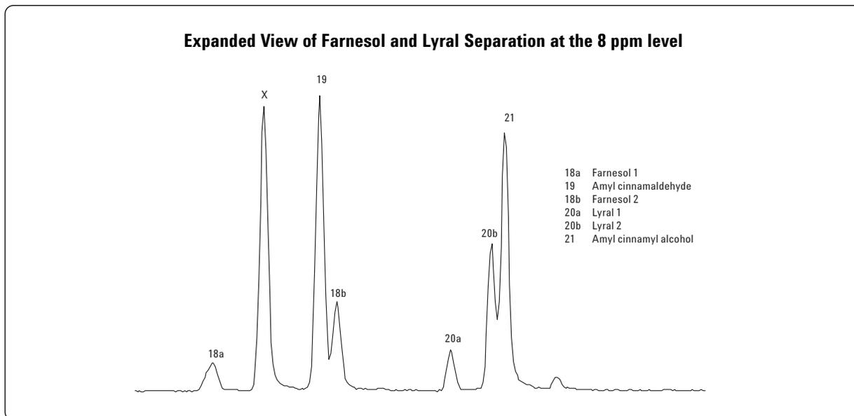
Figure 2. Expanded view of farnesol and lyrals separation at the 8 ppm level on a Agilent J&W DB-17ms, 30 m × 0.25 mm, 0.25 μm column (p/n 122-4712). GC conditions used are in Table 1. The x label peak is a contaminant present in the 24-allergen mix and not an analyte of interest.
