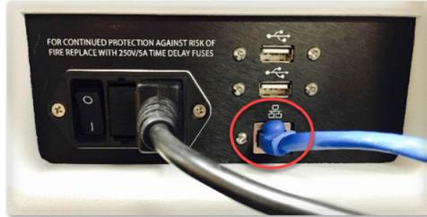
Figure 4. Ethernet port with wired network connection cable
