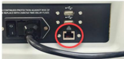
Figure 3. Ethernet (RJ-45) jack location outlined in red
