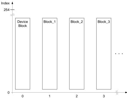
There are 254 indices per slot. The indices can have a width of 255 bytes. All values that can be accessed via Profibus have to be mirrored to one of these slots/ indices.
