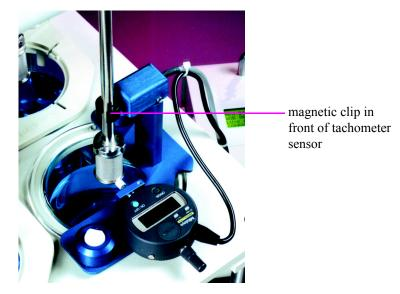
Figure 12 Placement for RPM Reading, Basket
