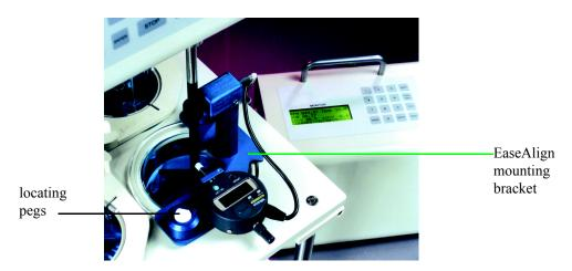
Figure 11 EaseAlign Mounting Bracket Secured to Dissolution Apparatus
