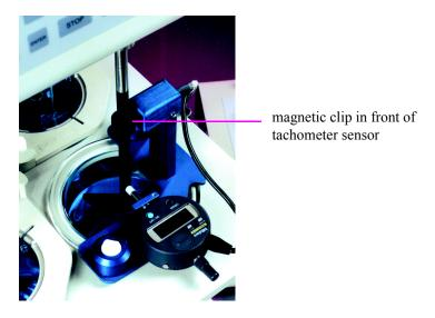
Figure 15 Placement for RPM Reading, Paddle
