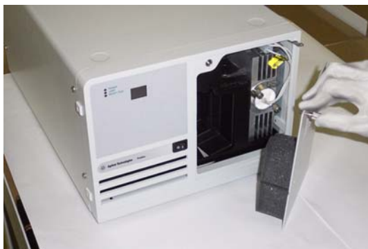
Figure 13 Removing the front panel
