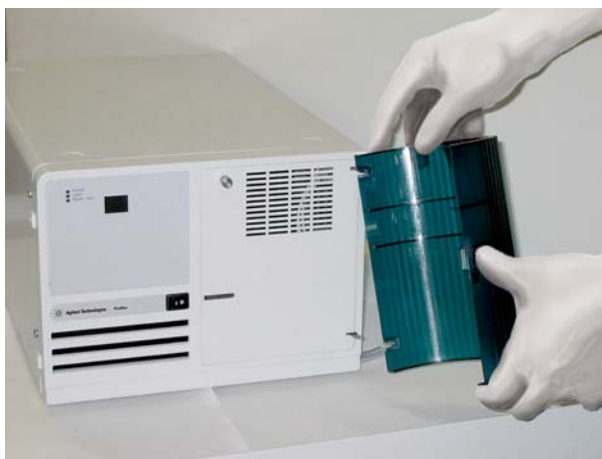
Figure 15 Installing the Agilent 325 Detector door
