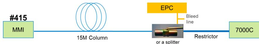
**G3445B-#412:** Fast Constant Flow (CF) method: 20-min run, 15 m column x 15 m column, mid column backflush.
