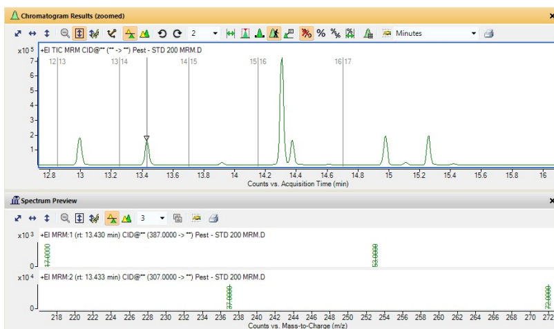
Figure 18 Walk chromatogram to view the two MRM spectra for the peak at 13.43 minutes
