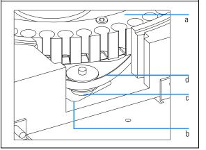
Put roller plate on top of foam (a).Make sure the three holes fit correctly (b).Use a knife to cut away overlapping foam.
