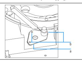
4 The new cut-out must look like this (a). Remove all foam cuttings. Remaining cuttings inhibit proper function.
