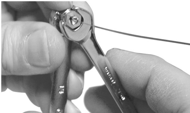
Figure 3 Tightening the swaging nut
