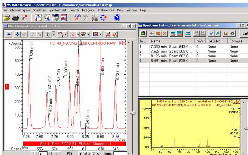
A spectrum list can also be generated by selecting **Spectrum List > Build Spectrum List From Active Chromatogram** in the MS data Review menu. This command opens the **Edit Integration Parameters** dialog.
