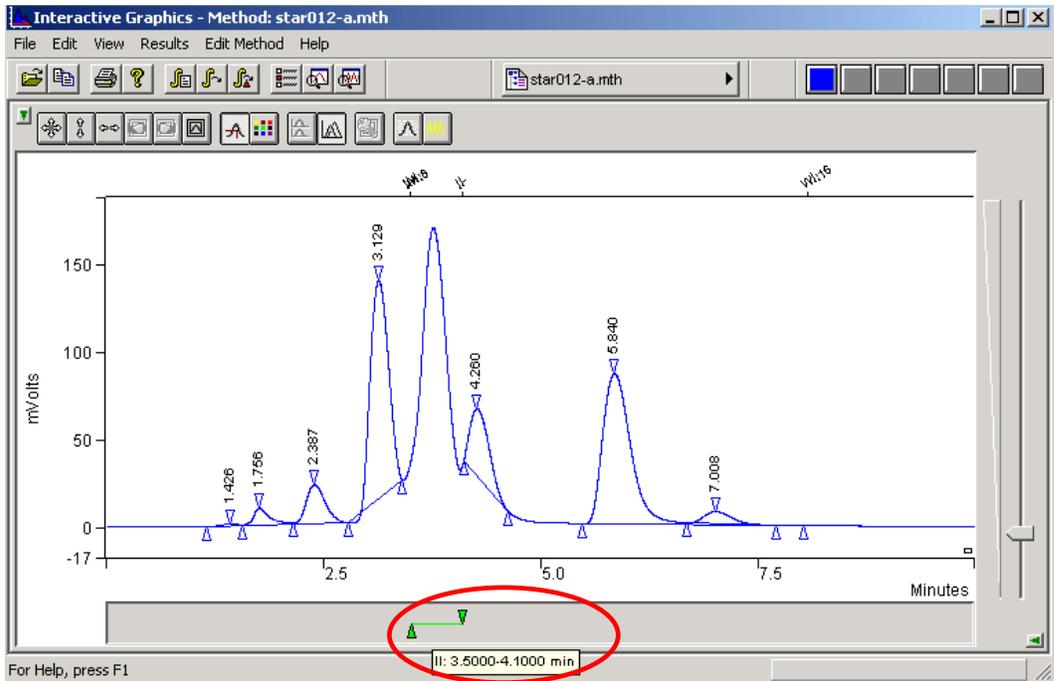
You can move the II event by clicking and dragging the triangles marking the start and end times.
