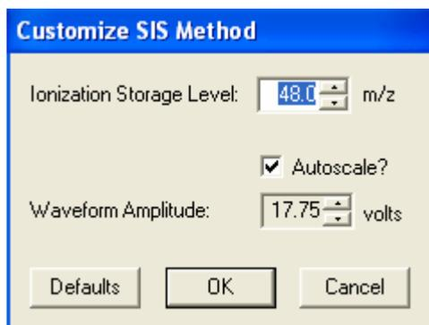
This selection will assure that optimum waveform amplitude is calculated, which will eject all the ions except the ones selected for storage. You can further optimize the waveform amplitude value by adjusting the **SIS Amplitude Adjust Factor** in the **Auto Tune** mode in **System Control** as will be described later in this tutorial. Save the method file as CalSIS by using the menu command **File > Save As** and then close the **Method Builder** application.
