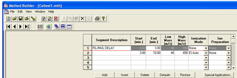
The default table for a new MS section consists of two segments. The first segment is a Filament/Multiplier Delay segment for the first three minutes (ionization Mode = None). This segment will be acquired with the filament and multiplier turned off to protect the instrument until after the elution of the solvent peak.
