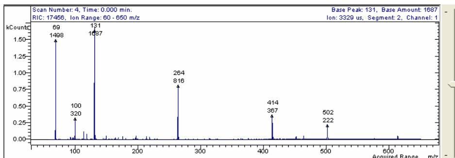
The waveform amplitude value is too low (50% of the one calculated by choosing Autoscale) and as a result the unwanted ions are not ejected effectively. Note that the base peak ion is 131 and its intensity is lower compared with the base peak intensity in the first spectrum due to the fact that EI Auto sets an optimum limit in the total number of ions stored in the trap.
