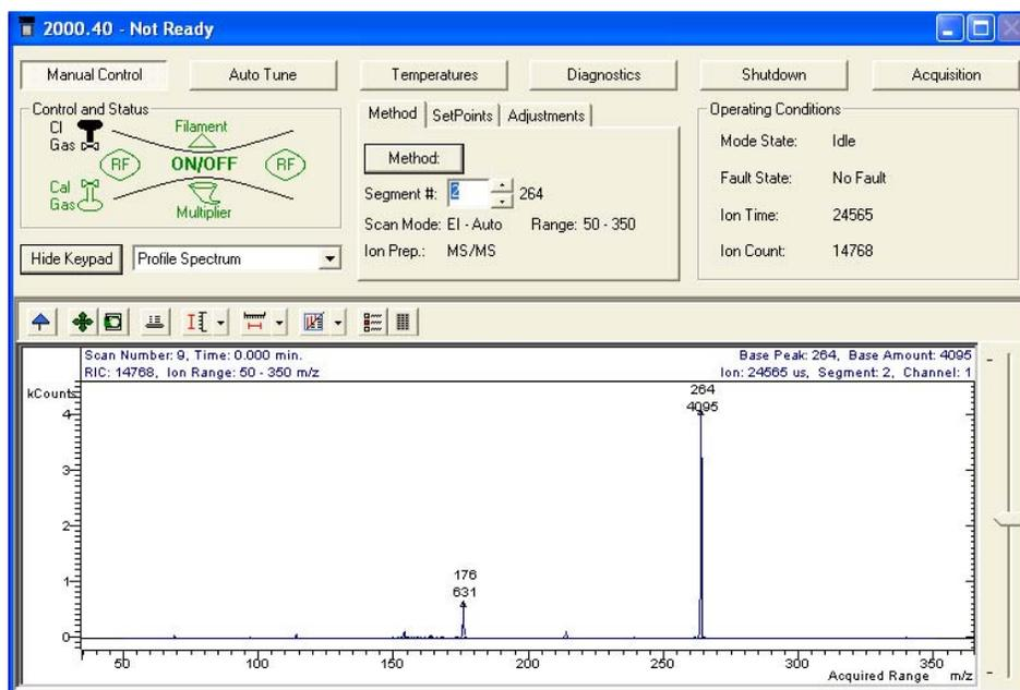
The  $m/z$  264 peak is still large, the Excitation Amplitude can be increased more. Set the Excitation amplitude to 50 and repeat the steps described above to acquire the mass spectrum.
