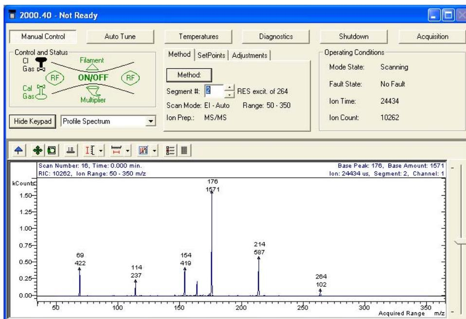
If the  $m/z$  264 peak is small and the product ions are visible:  $m/z$  214, 176, 164, 154, 114, the voltage will be a good one to use. For this ion trap system, the optimum value of the Excitation Amplitude is 0.5.
