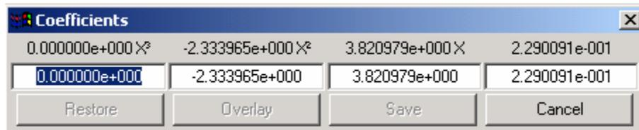
Click on the **Overlay** button in the **Coefficients** window to compare curves for the two sets of coefficients.
