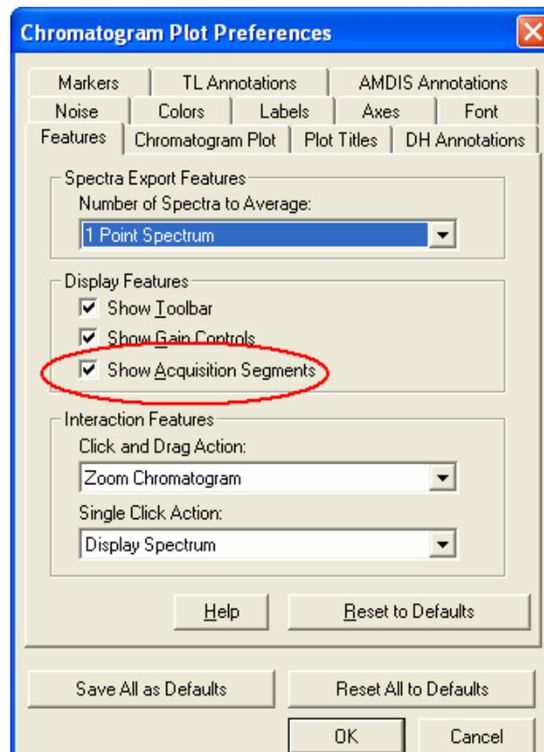
A graphical representation of the acquisition segments is displayed at the bottom of the Chromatogram window.
