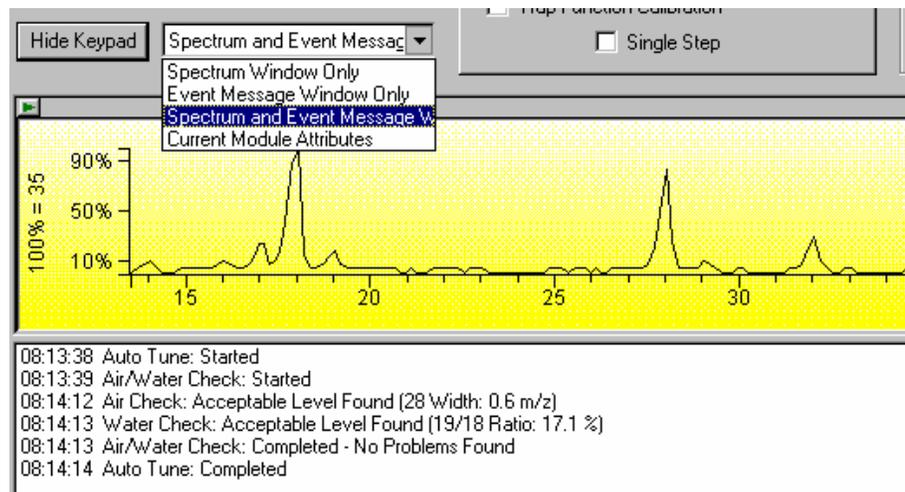
When the Air/Water check completes, the Multiplier Tune and Mass Calibration methods will be run automatically unless you have selected “Single Step” in the checkbox below. In “Single Step” mode, the tuning will pause between Auto Tune steps so that you may examine the results of each test and then click the **Continue** button in the Status and Control field to initiate the next Auto Tune procedure.
