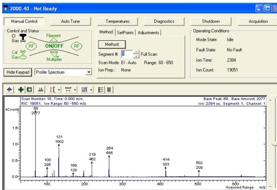
The mass spectrum displayed in the above picture was acquired with segment 1. It shows all ions in the calibration gas, as there is no ion preparation selected. Select the second segment that uses the SIS ion preparation to store only the m/z 100, 264 and 414. The mass spectrum acquired with segment 2 (SIS on) shows only the selected ions.
