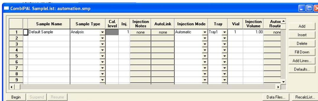
Add the samples you wish to run to this list. Type in sample name and vial position information for your samples. Use the pull down arrow to select Analysis under Sample Type.
