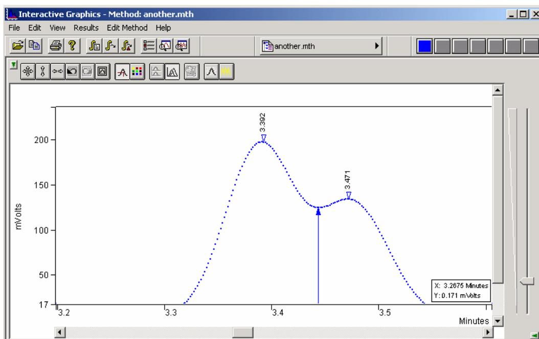
Note that the peak event triangle for the valley point is now drawn as a solid triangle indicating a moved peak event. Now that the point is repositioned, you can recalculate the file using the moved baseline event.
