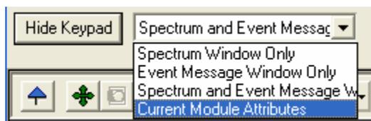
The Current Module Attributes section of the display shows the current settings and tune status of the instrument. This information is also added to the Segment Log for all acquired data files. Therefore, you can verify before a run, or in examining past archived data files, that the instrument tune is valid.
