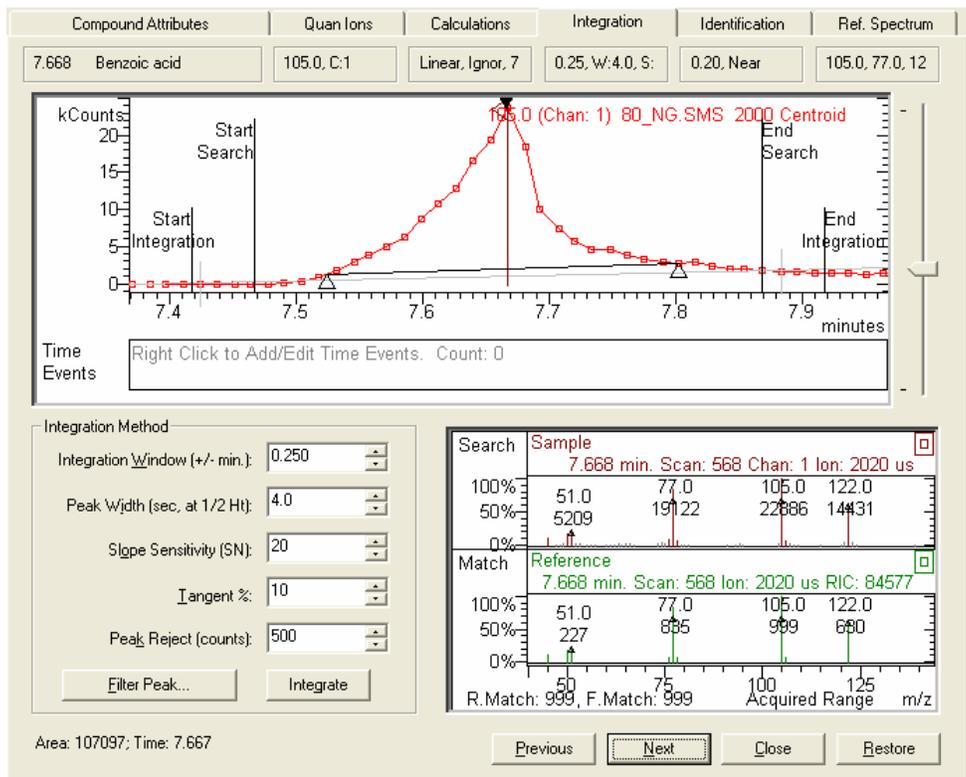
Benzoic acid is integrated, but the segment end point is too high. Increase the Peak Width parameter. You will discover that this parameter alone does not allow good control for moving the ends of the segment defining the integration region. When you increase the Peak Width up to 16 sec, both point ends are moved, but they are too far out. Increase the Slope Sensitivity parameter from 20 to 160 and integrate again.
