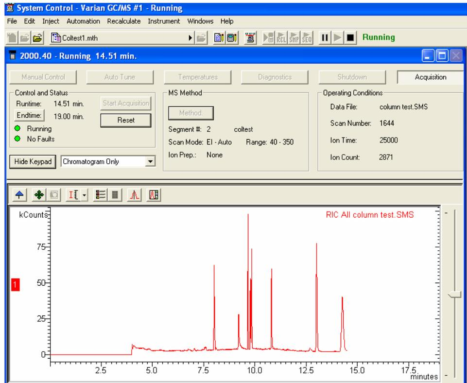
When the Runtime reaches 4.0 minutes, Segment 2 will be downloaded and acquisition will switch to EI-Auto mode. Again note the information displayed in the MS Method and Operating Conditions regions. Move the mouse over the buttons in the display toolbars and examine the options available. Choose the
