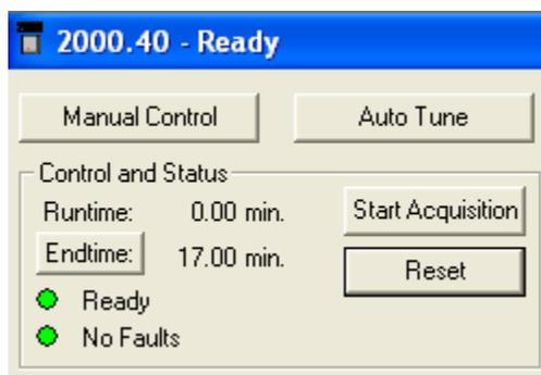
You may also use the **Windows** menu to check the status of the GC module as well. While the GC injector and column temperatures are being adjusted to those set in the method, the GC module status will be “Equilibrating”.
