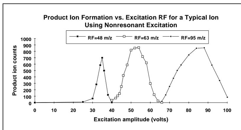
The maximum production of product ions shifts to higher CID (excitation) amplitudes as the excitation storage level is increased.
