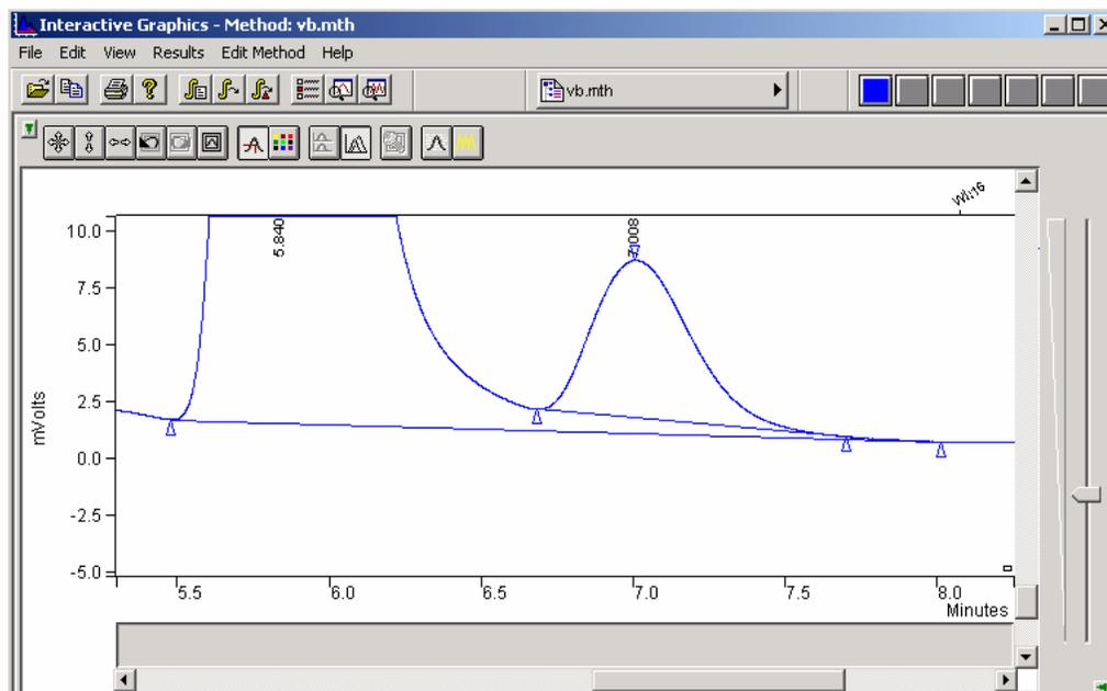
The current Tangent Height Percent threshold is 10%. Notice that, at this setting, the peak at 7 minutes is skimmed as a tangent peak.
