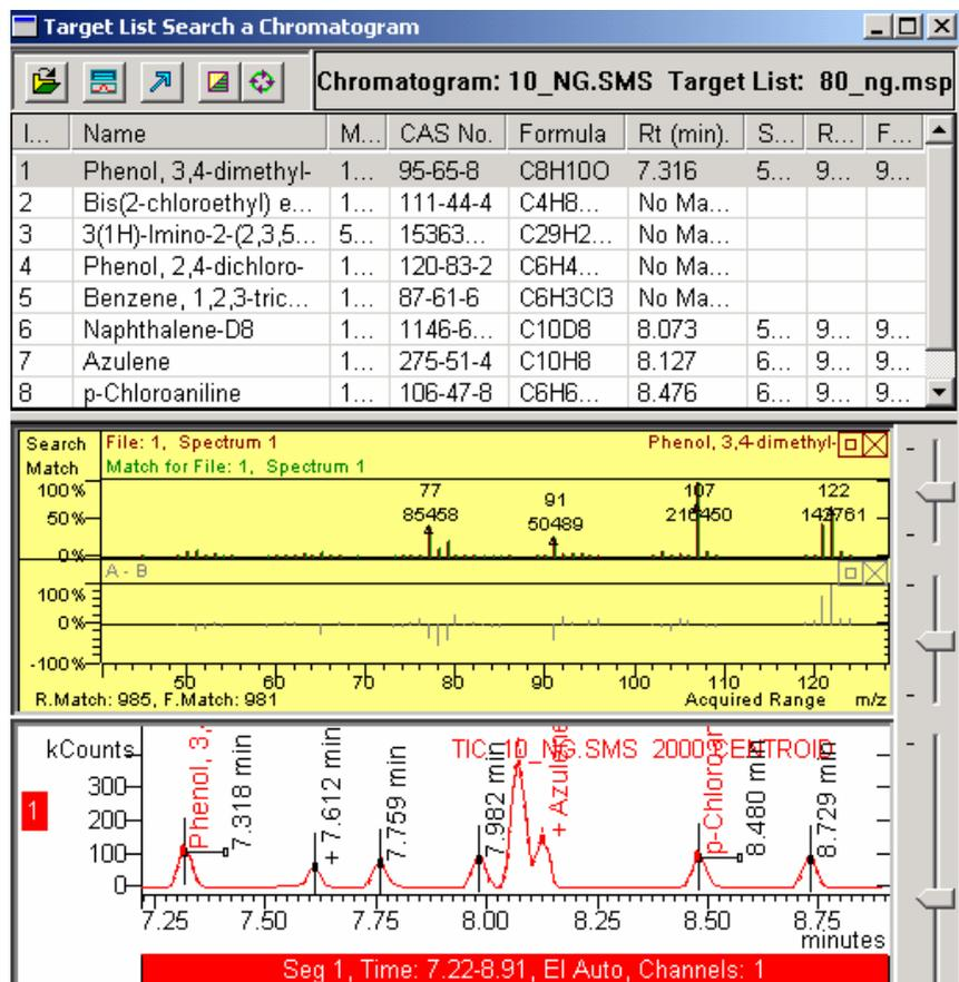
Highlight a peak in the list and observe the mass spectrum and the peak location in the displays below. Use **Next** and **Previous** buttons to navigate the list.
