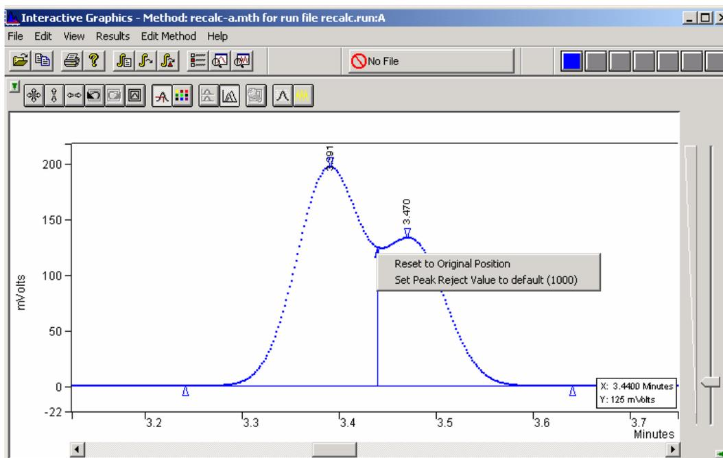
If you reintegrate now after restoring the valley point to its original position, you should get the initial integration results. After examining the reintegration results, close the Results window.
