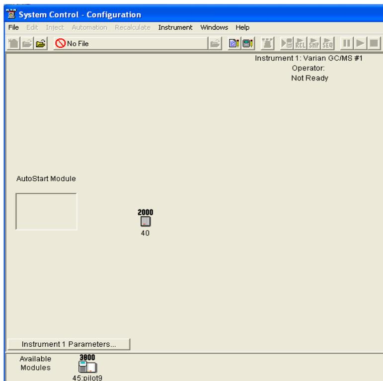
If you have a 8200 AutoSampler, drag and drop the Autosampler icon to the Available module area (note that the CP-8400/8410 is controlled and displayed through the GC Status and Control screen; it requires no special treatment). This removes the GC and the AutoSampler modules from the instrument, and the methods is not downloaded when an MS method is activated. To restore the GC and Autosampler modules, move the icons back into the active field.
