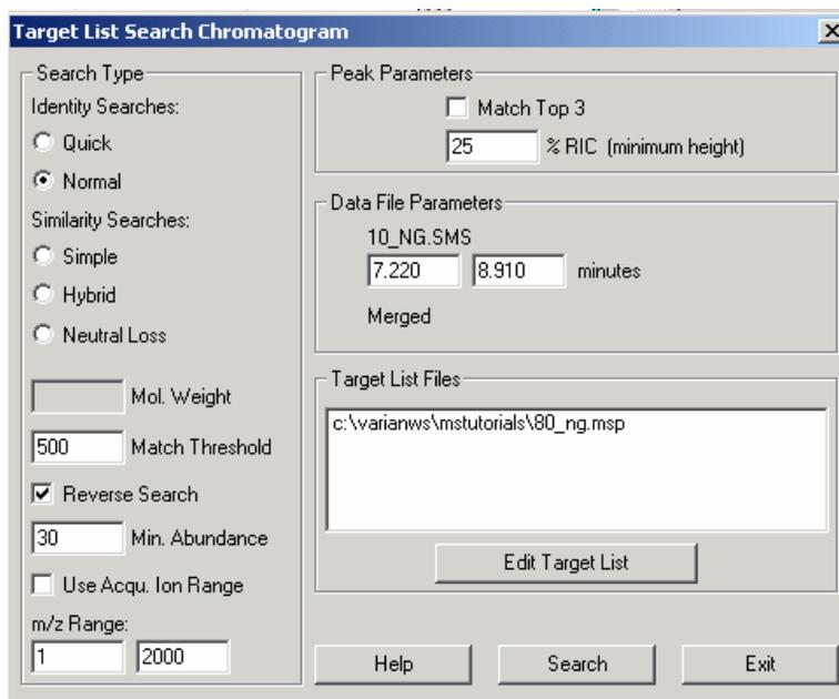
In the Target List Files click the **Edit Target List** button. This will open the **Spectrum List Manager** dialog from which you can select the list(s) used to search the chromatogram.
