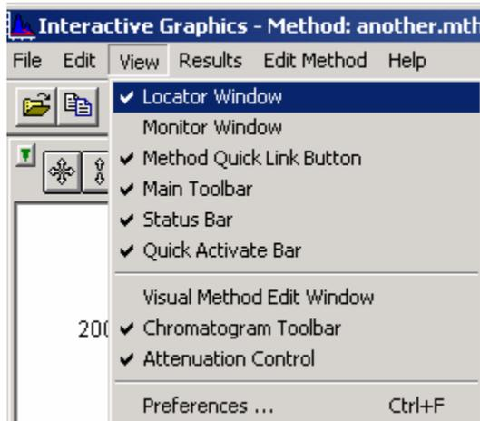
Now, zoom in on the center of the fused peak eluting at about 3.4 minutes. To zoom, highlight the desired area in the locator window or highlight the region in the main window from 2.5 to 4.0. (Areas of the display can be highlighted by clicking on the upper left hand corner of the region you wish to zoom with the left mouse button, dragging the mouse to the lower right hand corner of the area you wish to display, and releasing the mouse button.)
