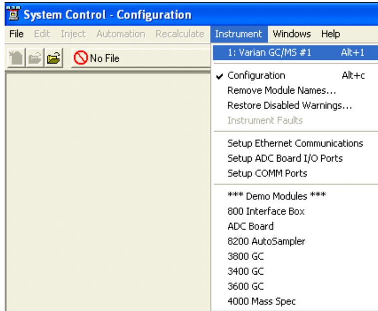
The window titled “System Control - Varian GC/MS #1” will appear. The 2000 Module Window appears directly within it. If it is iconized, double-click to open it. There are six different modes of operation. By default, the Manual Control mode is active when you enter System Control. Other screens will appear when Auto Tune, Temperatures, Diagnostics, Shutdown, and Acquisition buttons are clicked. Note that the System Control and 2000.40 (2000 MS module) title bars both show **Not Ready**.
