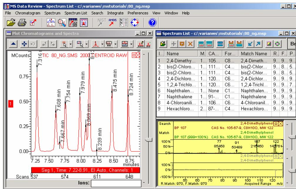
Use the up and down arrows to highlight entries in the table and to examine the mass spectra. Note that you can adjust the splitter bar separating the display areas to size the fields to your preference.
