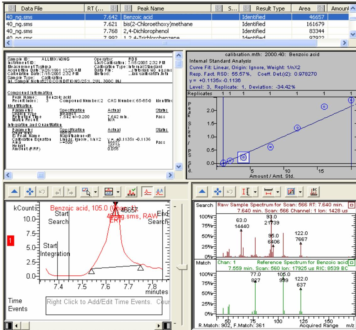
In the Results view you can examine the calibration and analysis results and interactively adjust the integration parameters for any compound in any data file, which you select from the list displayed on top of the Results view.
