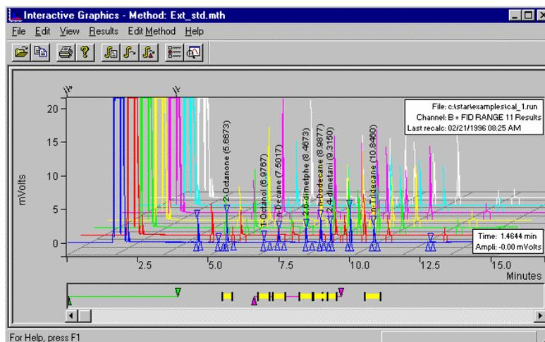
Next, you will load the method file which will be used for the analysis. You will use the method file, INT\_STD.MTH, located in the ChromExamples directory. The information in the peak table is necessary to generate the coefficients of the calibration curve.
