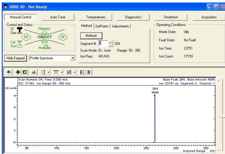
If the  $m/z$  264 is the only ion in the mass spectrum, a higher voltage is needed to dissociate  $m/z$  264. Click the **Method** button, increase the Excitation Amplitude to 40, save the changes and reactivate the method. Turn on the trap and the calibration gas and observe the spectrum.
