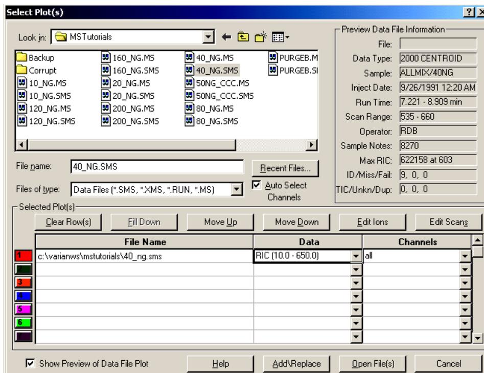
After selecting a file, click **Add\Replace**, then **Open File(s)**. The RIC (Reconstructed Ion Current) is displayed if RIC was selected in the Data column. To display chromatograms generated by specific ions, see the topic “How to Display Mass Chromatograms” below.
