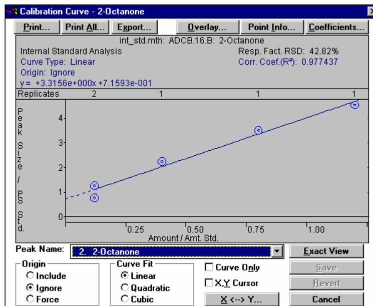
The Y axis of the calibration curve represents the ratio of the peak size of the analyte compound to the peak size of the internal standard. The X axis represents the ratio of the amount of the analyte compound injected to the amount of internal standard injected.
