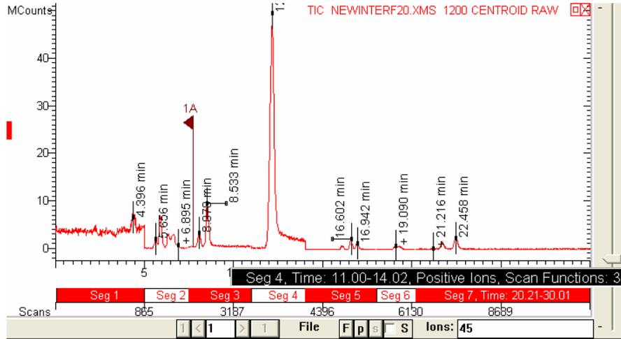
If multiple plots are displayed, the Segments control refers only to the active plot. Click on or below the segment bar in the chromatogram plot. The **Data File Information** window will be opened.
