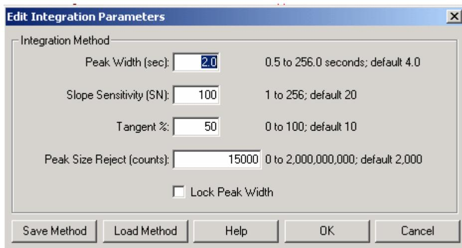
Press the **Help** button in the **Edit Integration Parameters** window to find the significance of the fields and buttons in this dialog and how are they used to make a spectrum list. Use the default values and press **OK**. The spectrum list is displayed as well as a spectrum window for visualizing each spectrum in the list. Explore the influence of different integration parameters values in the peak detection process performed to build the list.
