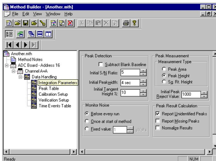
The **Integration Parameters** window opens, showing the current settings. Peak measurement is by height, and Report Unidentified Peaks is checked.
