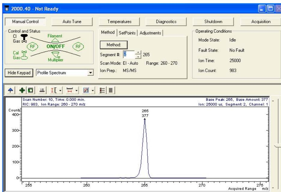
The  $m/z$  265 ion has been isolated but its peak intensity has also been slightly reduced due to the fact that the isolation window has become too narrow by decreasing the Low Edge Offset value to 2.
