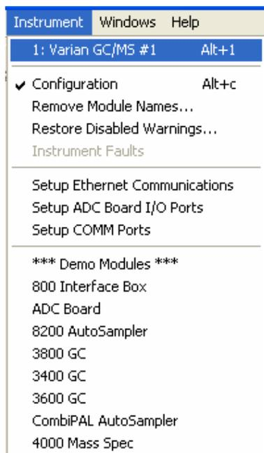
Activate the method that you are going to use for the AutoSampler, GC and MS using the menu command **File >Activate**, select the method and then click **Open**.
