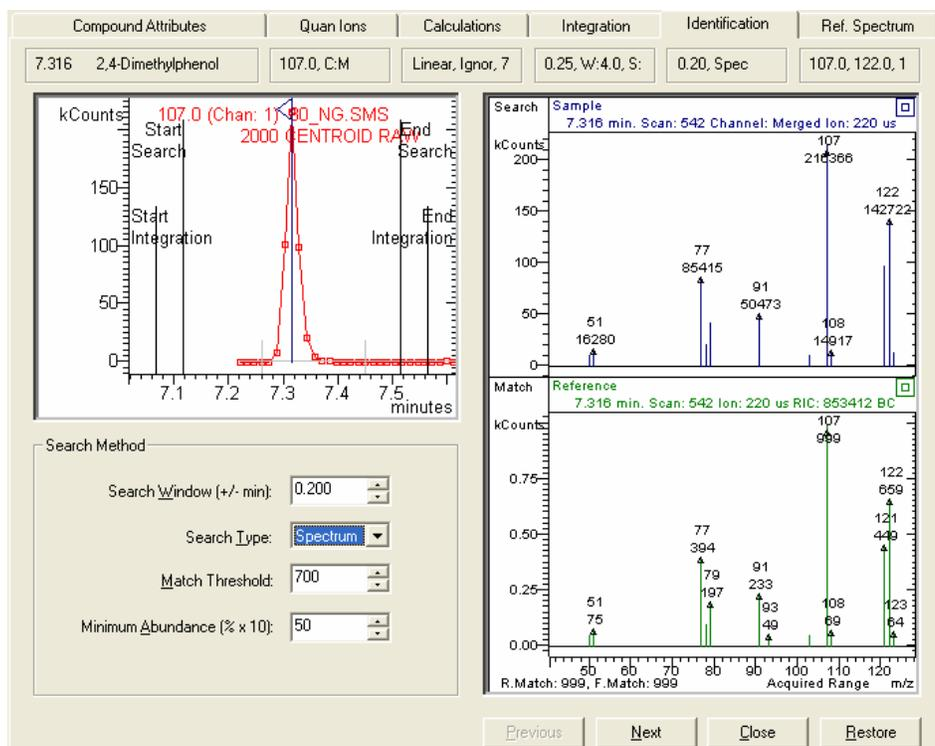
You can use the default Identification parameters for all peaks in the Compound Table except for benzoic acid. For this peak, enter a peak width of 0.400 min.
