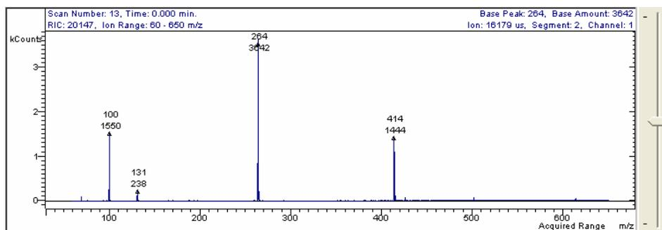
The base peak ion is 264 and its intensity increased, however the ejection of the 131 ion is not complete.
