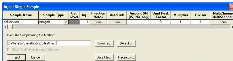
The active method is displayed in the field **Inject the Sample using the Method**. Type in a name for your sample in the **Sample Name** field. Here we have just chosen the name column test. After typing the name, you can activate the **Data Files** button by clicking in any other field. Click on the **Data Files....** button to open the **Data File Generation** dialog.
