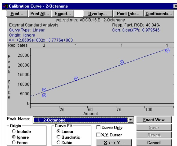
The Y axis of the calibration curve corresponds to peak size. The X axis represents the amount of the compound injected.
