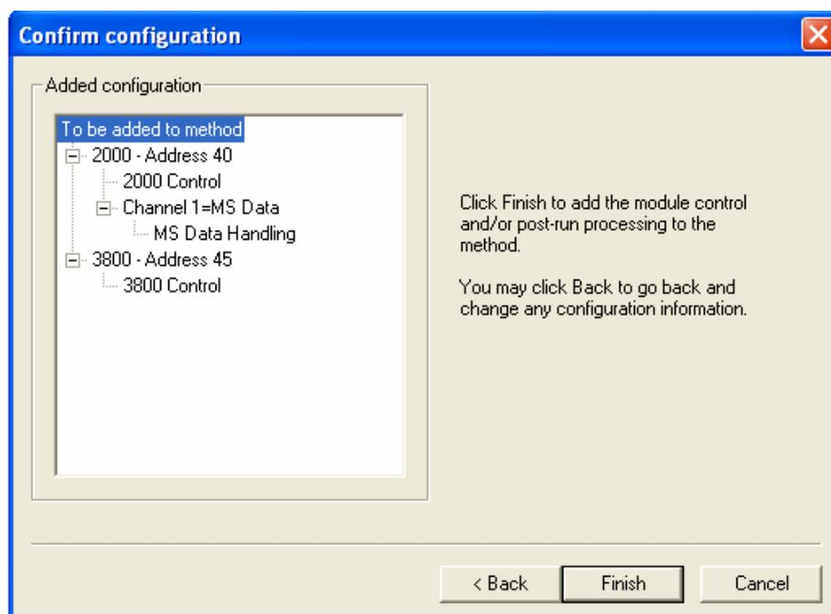
The **Confirm Configuration** dialog shows that you will create the new method with sections for 3800 GC control and 2000 MS control.
