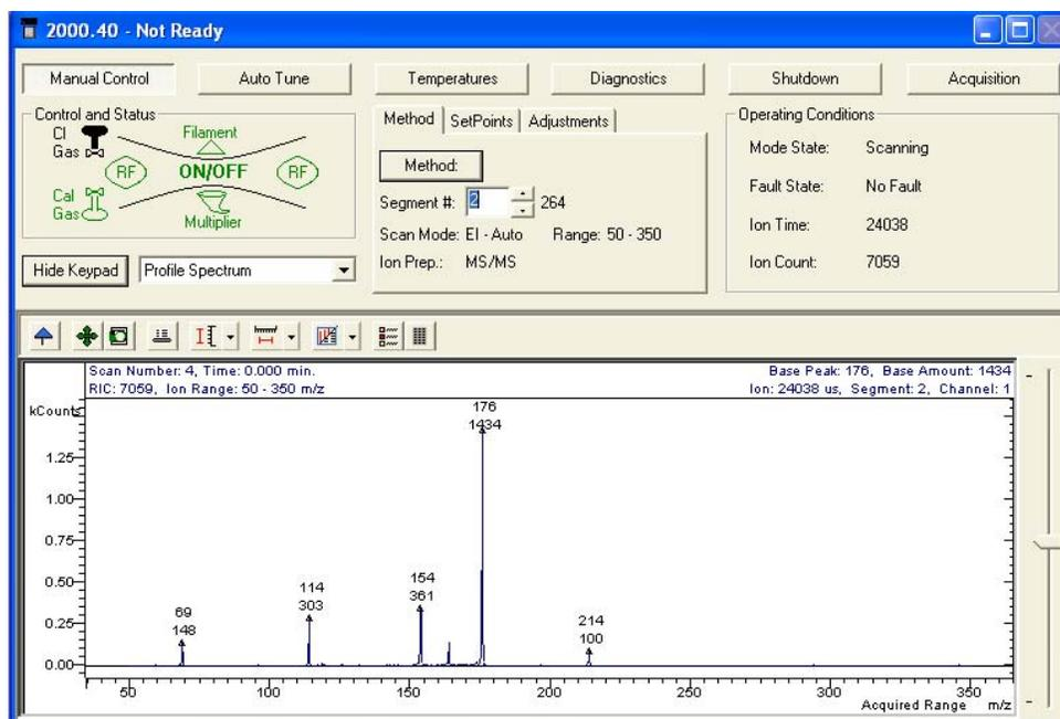
The parent ion  $m/z$  264 is totally absent. You may choose an intermediate value of 45 for the Excitation Amplitude. If the  $m/z$  264 peak is small and the product ions are visible ( $m/z$  214, 176, 164, 154, 114), the voltage will be a good one to use. Set the Excitation Amplitude value to 45 and record the mass spectrum.
