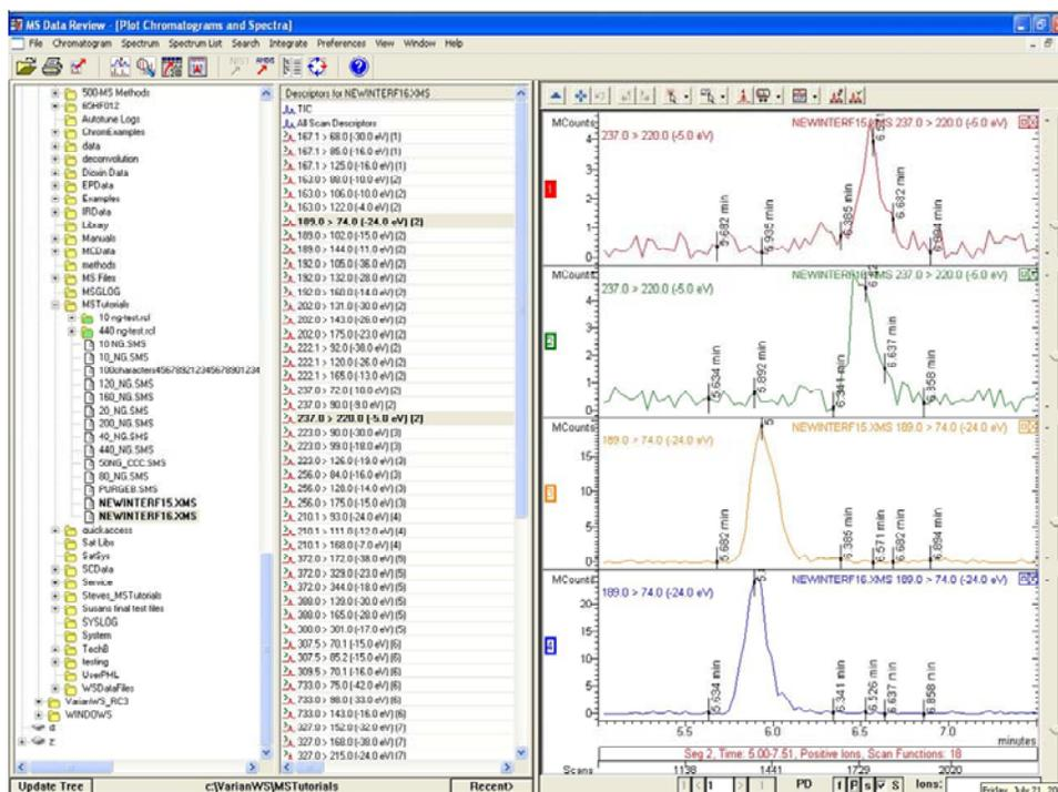
6. Use the
