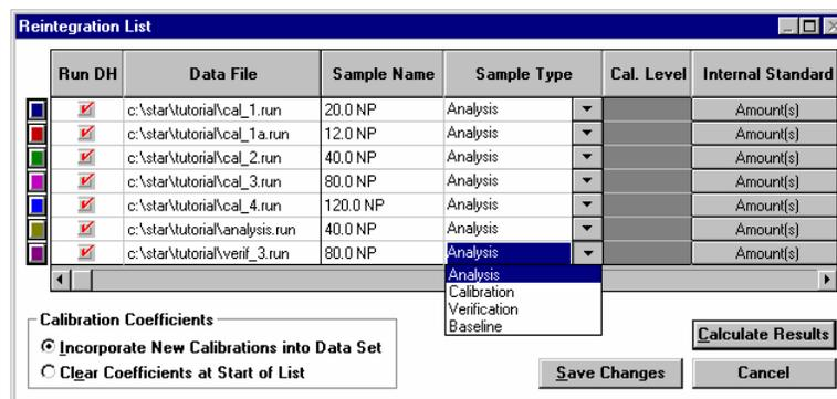
The data file for each chromatogram displayed in IG appears here. The fourth column in the Reintegration List is the Sample Type, which must be set as Calibration for the first five files, Analysis for the sixth and as Verification for the last one.
