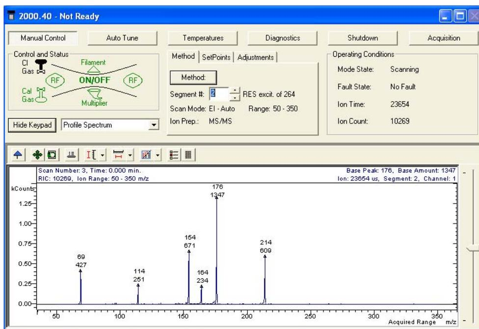
If the  $m/z$  264 peak is absent and only the product ions are visible ( $m/z$  214, 176, 164, 154, 114) with smaller peaks than before, the excitation voltage is too high. If only the  $m/z$  264 peak remains, try increasing the modulation range in the **Customize** dialog.
