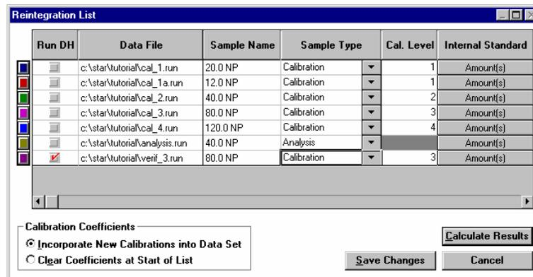
After processing has completed, the data from VERIF\_3.RUN will have been added to the previous calibration set. All curves will now show two replicates for level 3.
