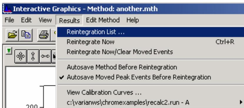
The **Reintegration List** dialog opens. A check mark appears in the Run DH column for the data file. This indicates that the file is selected for recalculation.
