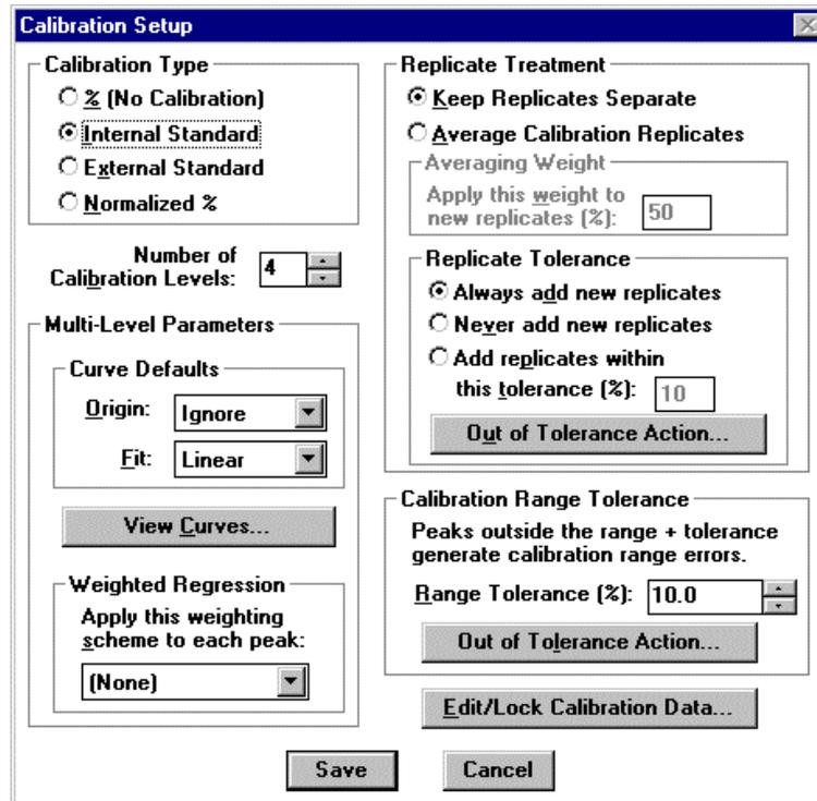
The Calibration Type should be Internal Standard. The Number of Calibration Levels should be set to 4. The Curve settings should be Linear, Ignore.
