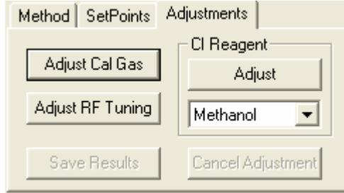
If the RF Ramp is not passing test requirements, open the front door of the MS and find the labeled RF Adjustment screw and adjust it with a flat-blade screwdriver while observing the feedback on the screen. When the Control and Status message reads "RF Response is Within Limits", click **Save**.
