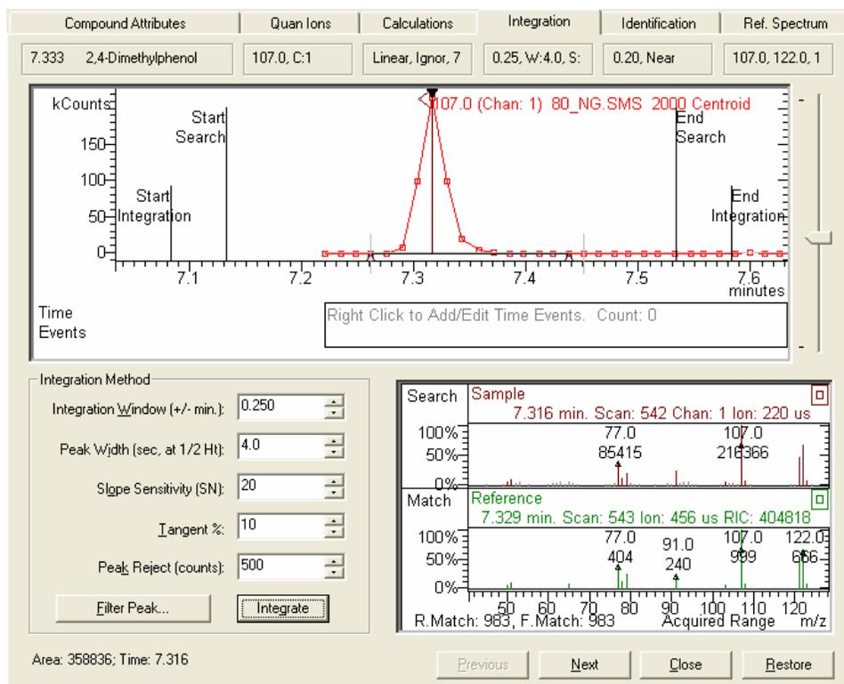
Check how the peak will be integrated by clicking the **Integrate** button. You will see the baseline drawn in the Chromatogram display and the peak area and retention time displayed to the lower left side of the Integration dialog. For this compound the integration process works well with the default integration parameters.
