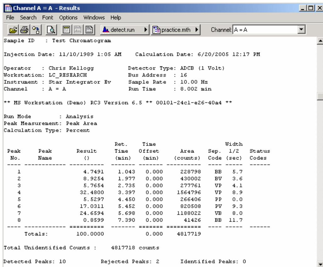
Compare this to the original results. You will notice that the retention times are slightly shifted and only 8 peaks are reported. The fused peaks at about 3.4 minutes are now reported as one peak. Also, only one peak was detected between 1.0 and 1.5 minutes. The total number of detected peaks is now 10.
