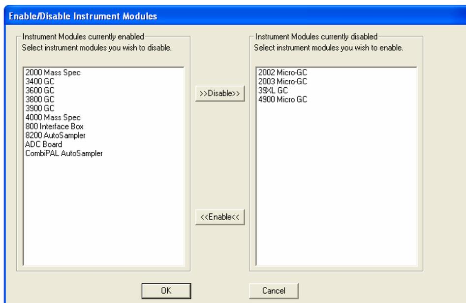
If for example you have a 3800 GC and a Combi PAL AutoSampler, enable the 3800 GC and the Combi PAL AutoSampler. (For users who have a CP-8400/8410 AutoSampler, the autosampler is controlled and displayed through the 3800 or 3900 Status and Control screen. Thus, only the GC needs to be enabled.) When the desired configuration is enabled, click on **OK** and open System Control.
