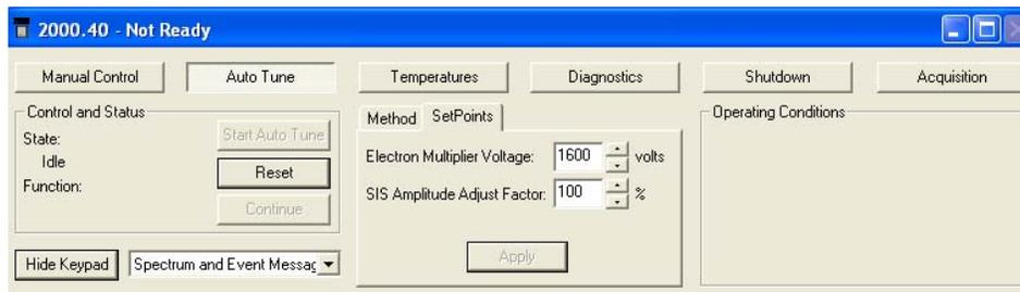
Set the SIS Amplitude Adjust Factor to 50 (the values may be set between 50 and 200) and acquire another spectrum with segment 2.
