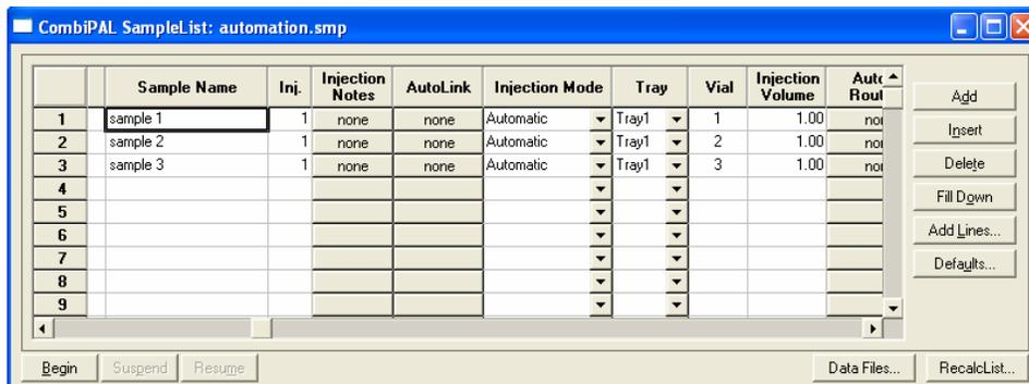
To start automation, click on the **Begin** button in the bottom left corner. The autosampler will inject the sample contained in vial position 1, followed by the samples in positions 2 and 3.
