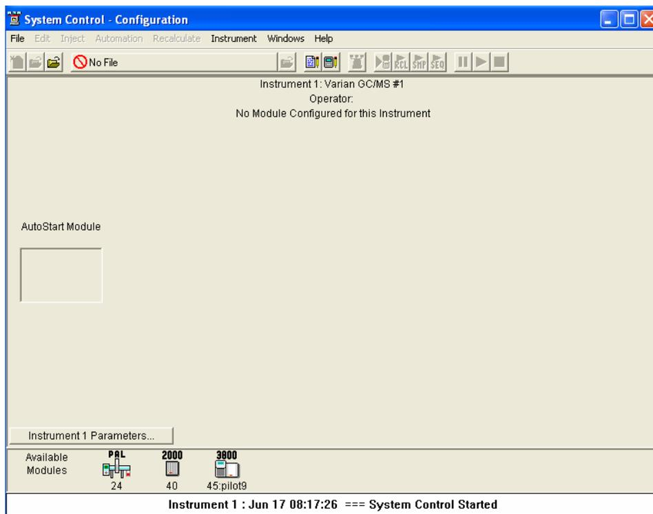
If the instrument has not been previously configured, the 2000, 3800 or 3900 GC, and the Combi PAL AutoSampler (if it exists in your system) will appear at the bottom of this screen in the “Available Modules” section of the window. Use
