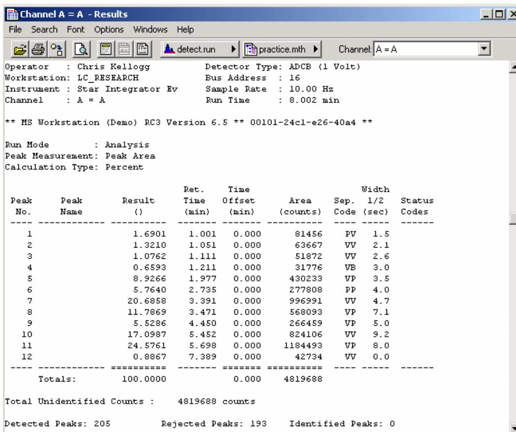
Now, the detected peaks correspond to all signals larger than the new S/N Ratio. The change in S/N Ratio affects the placement of peak events and baselines, the accuracy of which are necessary for reliable chromatographic quantitation. Setting the correct S/N Ratio is particularly important in percent calculations, where the results for each peak are expressed as a percentage of the total area or height counts for all the peaks.
