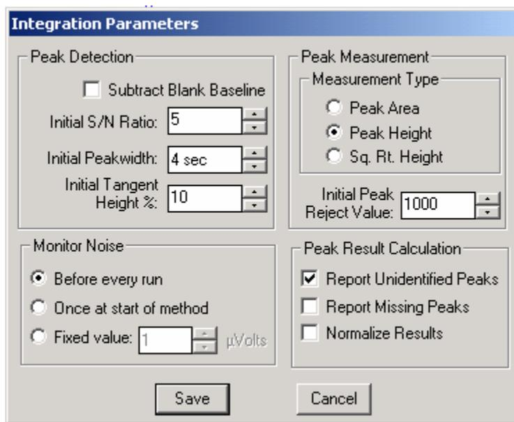
The Integration Parameters dialog box is partitioned into sections associated with the various functions of peak detection, measurement, and result calculation. Notice that the Results window is automatically hidden while you work on the method.
