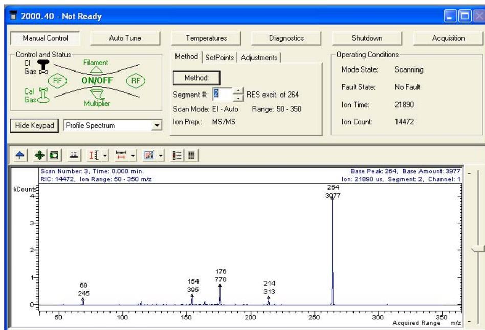
The height of the  $m/z$  264 peak should be reduced and several product ions should be visible:  $m/z$  214, 176, 164, 154, 114. The voltage may be further increased to convert additional parent ions into product ions. Set the Excitation Amplitude value to 0.5 and record the mass spectrum.
