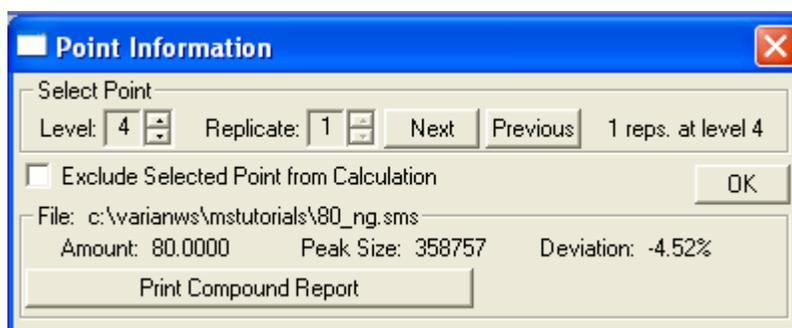
As you can see in the Calibration Curve plot, this data point has a greater deviation from the fitted line than other data points for the compound. Note the deviation value of  $-4.52\%$  in the Point Info dialog. Click on the box **Exclude Selected Point from Calculation**. Observe the change in the fit equation, response factor RSD, and the Correlation Coefficient when the point is excluded.
