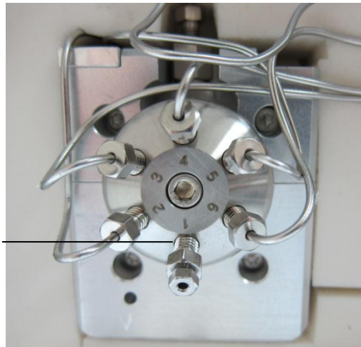
Valve port 1 with the Fitting-internal Reducer plugged
