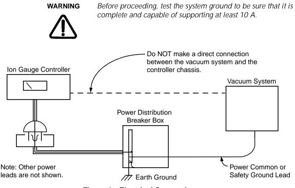
Figure 1 Electrical Connections
