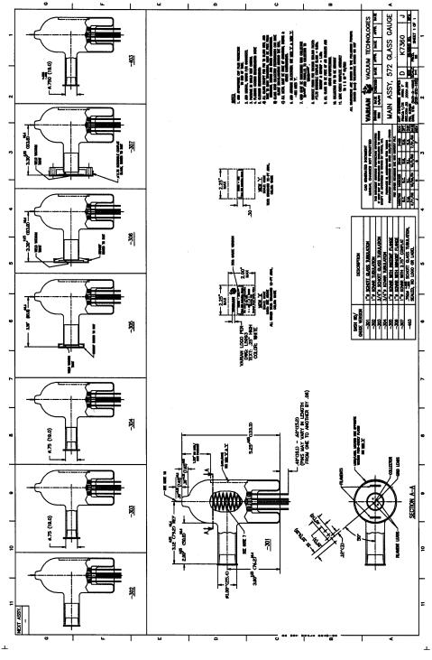
Figure 2 572 Ionization Gauge Tube Outline Drawing
