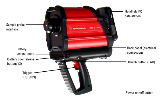
Figure 1. Agilent 4100 ExoScan FTIR
