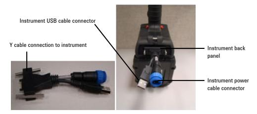
Figure 3. Power connections
