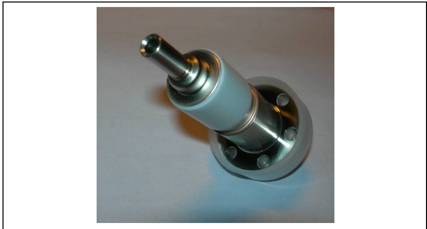
Figure 11 Ion pump feedthrough - OLD USA Connector
