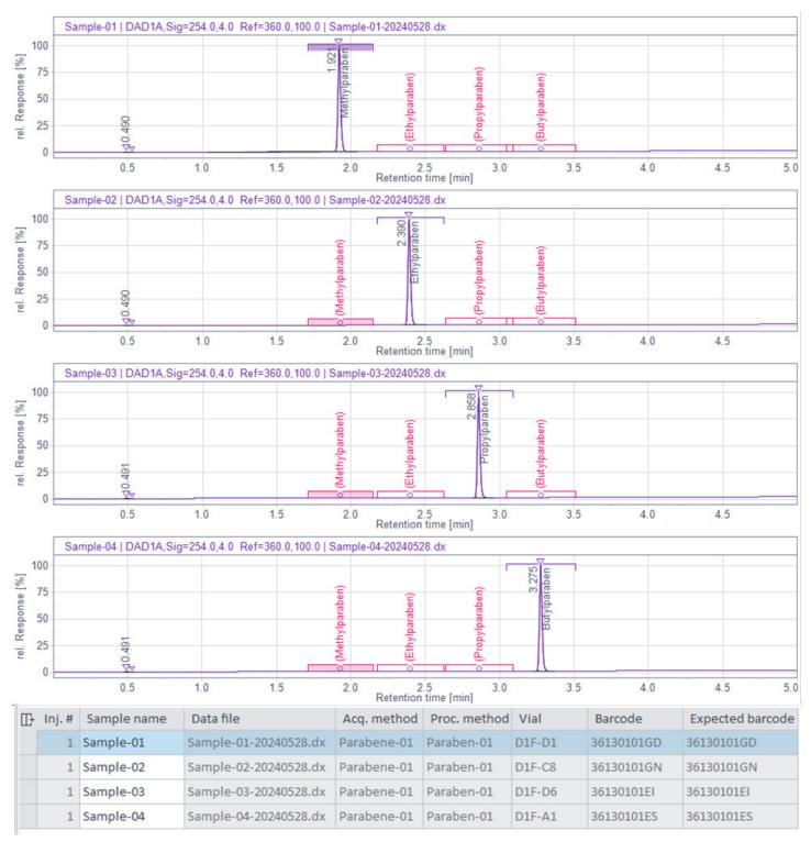
Figure 2. Identification of randomly placed samples by expected barcode. The expected barcode was introduced with the sequence table. The vial position was assigned after confirmation of the barcode by the Multisampler (vial label example: D1F-D1: Drawer1Front, position D1).
