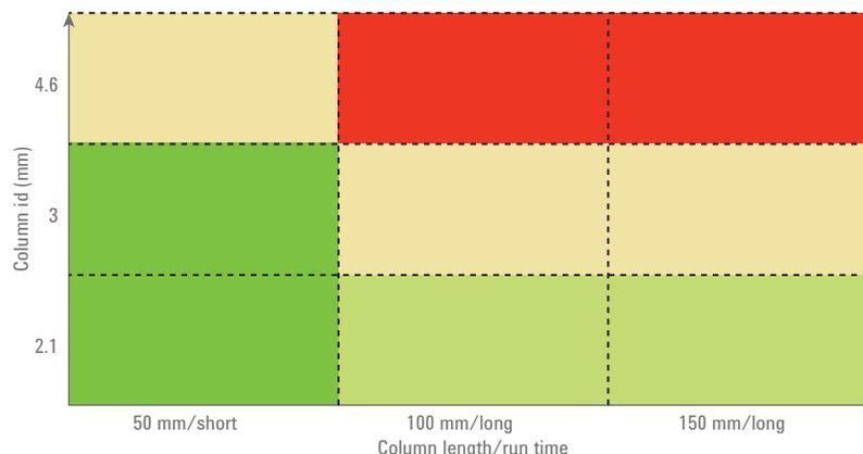
Figure 1. Overview improvements with ultralow dispersion kit for sub-2  $\mu\text{m}$  particle columns (dark green – highly recommended, light green – highly recommend for isocratic runs, yellow – conditionally recommended, red – not recommended).
