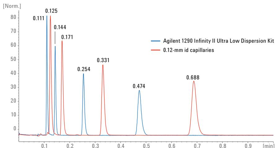
Figure 2. Isocratic separation of dimethylphthalate, diethylphthalate, biphenyl, and *o*-terphenyl using an Agilent 1290 Infinity II LC equipped with the Agilent 1290 Infinity II Ultra Low Dispersion Kit (blue), and a standard Agilent 1290 Infinity II LC equipped with 0.12-mm id capillaries (red).
