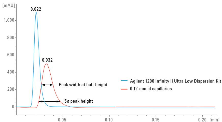
Figure 3. System dispersion measured at half-peak height and 5 $\sigma$  for caffeine. The measured system dispersion was compared to a standard Agilent 1290 Infinity II LC equipped with 0.12-mm id capillaries, and to a system from another vendor.
