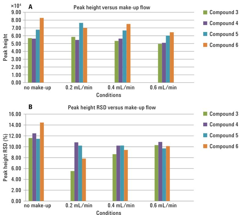
Figure 8. Peak height and peak height RSD % versus make-up flow rate at 30 °C temperature of a split SFC effluent. The peak height remained constant up to a makeup flow rate of 0.4 mL/min. The peak height RSD achieved a minimum at approximately 8 to 10 % for a make up flow rate of 0.4 mL/min.
