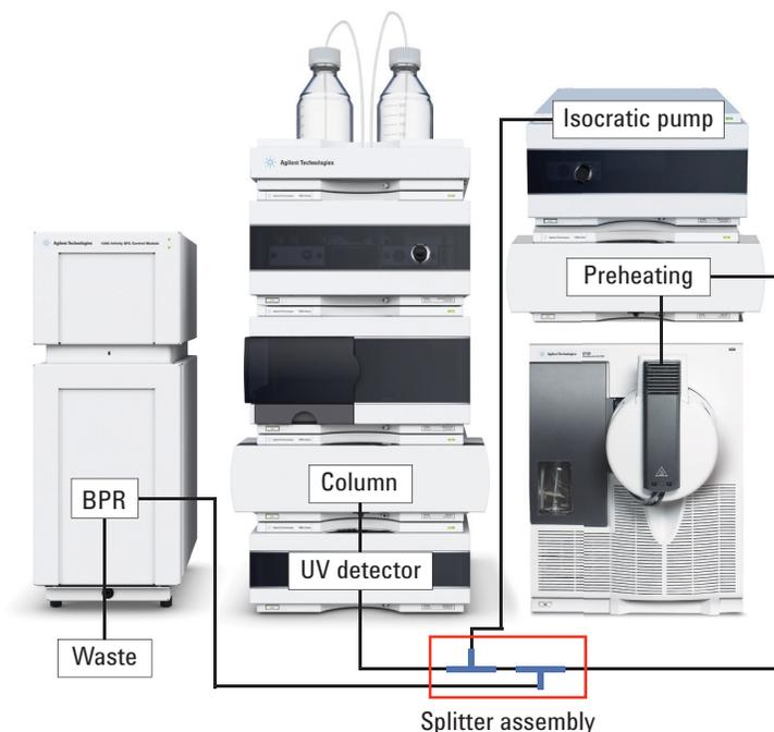
Figure 1. Configuration of the Agilent 1260 Infinity Analytical SFC Solution with the Agilent 6150 Single Quadrupole MS. The DAD flow cell is directly connected to the splitter assembly containing two splitters, a check valve, and a solvent filter (BPR = backpressure regulator, splitter assembly (p/n G4309-68715)).
