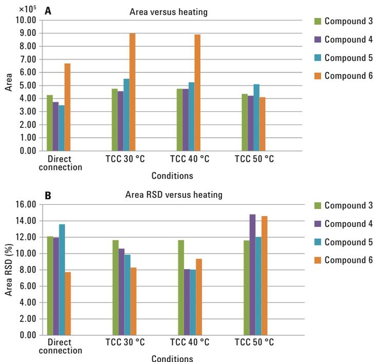
Figure 3. Peak area and peak area RSD % versus preheating temperature of split SFC effluent. The maximum peak areas were obtained at a preheating temperature of 30 to 40 °C with an RSD of approximately 8 to 10 %.
