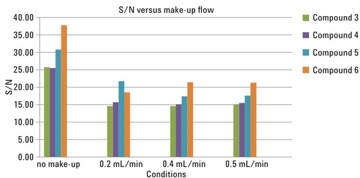
Figure 9. S/N ratio versus make-up flow rate at 30 °C temperature of a split SFC effluent. The S/N ratio, in comparison to the preheated example without make-up flow, decreased to a lower level when adding make-up flow, but remained constant for different make-up flow rates.
