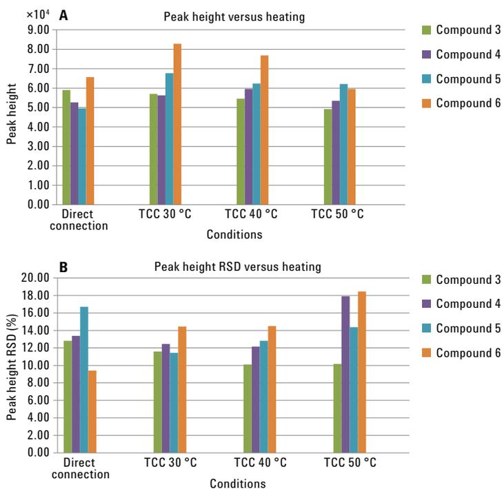
Figure 4. Peak height and peak height RSD % versus preheating temperature of a split SFC effluent. The maximum peak heights were obtained at a preheating temperature of 30 to 40 °C with an RSD of approximately 10 to 12 %.
