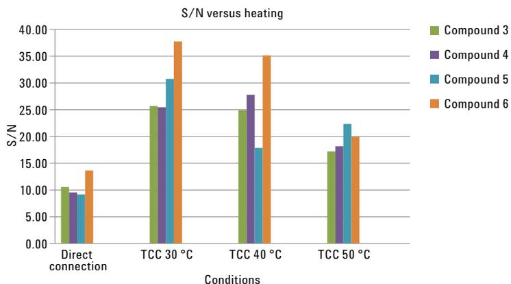
Figure 5. Signal-to-noise ratio versus preheating temperature of a split SFC effluent. The S/N ratios were at a higher level for a preheating temperature of 30 to 40 °C compared to direct injection.
