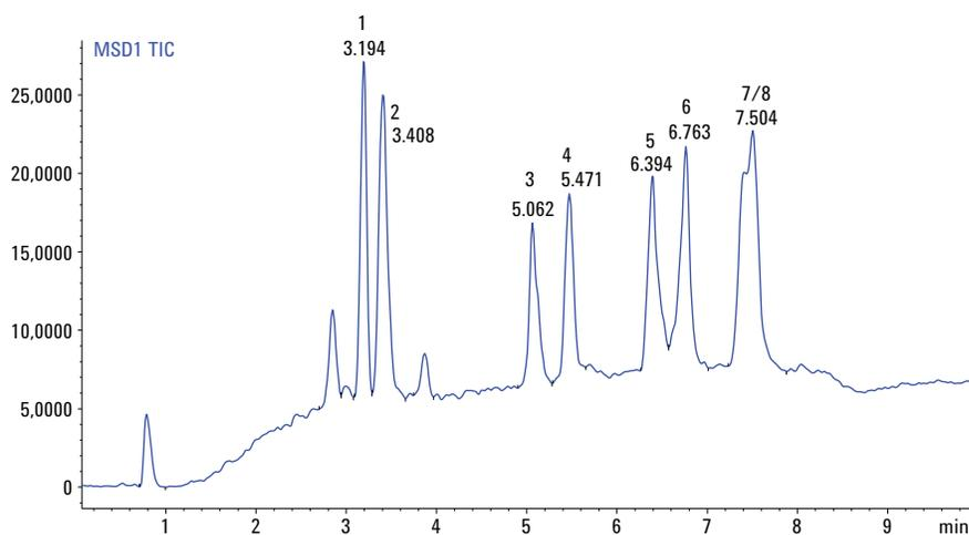
Figure 2. Separation of an eight-compound mix with SFC and single quadrupole MS detection. The splitting connection to the MS was located in the flow path behind the column and before the backpressure regulator by means of one T-piece of the splitter assembly and a 50 µm × 100 cm capillary.
