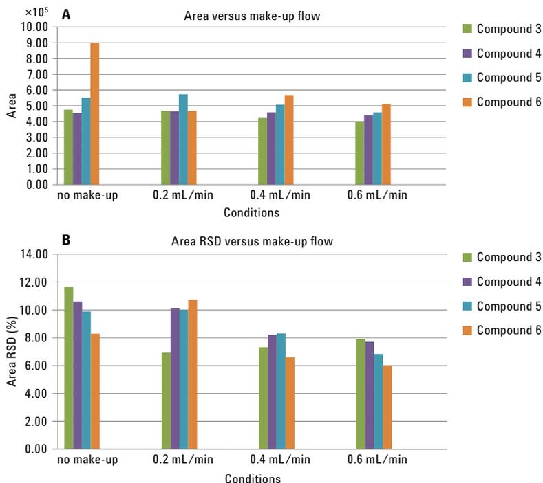
Figure 7. Peak area and peak area RSD % versus make-up flow rate at 30 °C temperature of a split SFC effluent. The peak areas were almost unaffected during the addition of a make-up flow but the area RSD achieved a minimal value at approximately 6 to 8 % for a make up flow rate of 0.4 mL/min.
