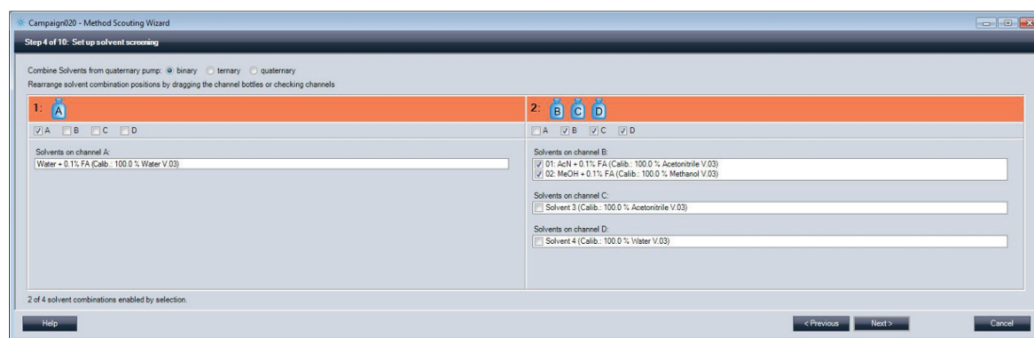
Figure 5. Solvent selection with a quaternary pump, which was used in binary mode to combine the solvent at channel A and one of the solvents at channel B.
