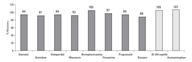
Figure 3 Compound fractionation on the Agilent SampliQ SCX cartridge. Neutrals (light grey bars) elute exclusively in the methanol step. Capture of the methanol eluent provides a means of characterizing neutral compounds separately from the basic compounds. Likewise, basic compounds (dark gray bars) are exclusively isolated in the methanolic ammonium hydroxide eluent.
