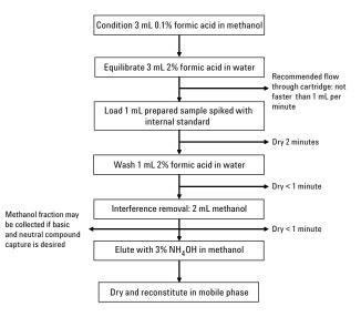
Figure 2. Agilent SampliQ SCX method development process for 3-mL cartridge.
