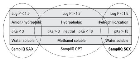
All of Agilent's polymer phases exhibit mixed-mode behavior. For SampliQ SCX this characteristic results in one cartridge which is useful for both neutral and basic compound separation.
