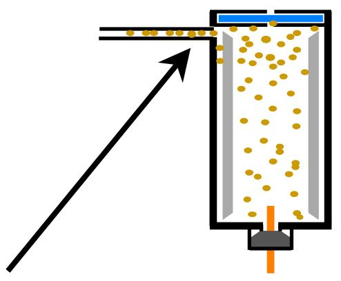
Sample expands to overfill injector liner and injection port Some sample condenses on cooler areas (bottom of septum, metal body, etc.) leading
