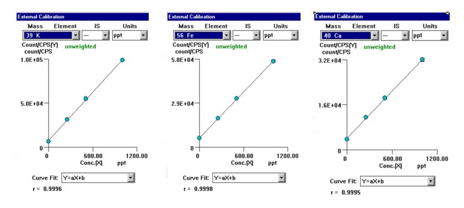
Elimination of Ar and ArO interferences on K, Ca and Fe respectively.
