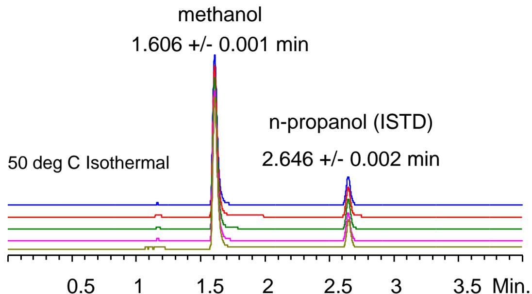
Methanol retention time standard using
