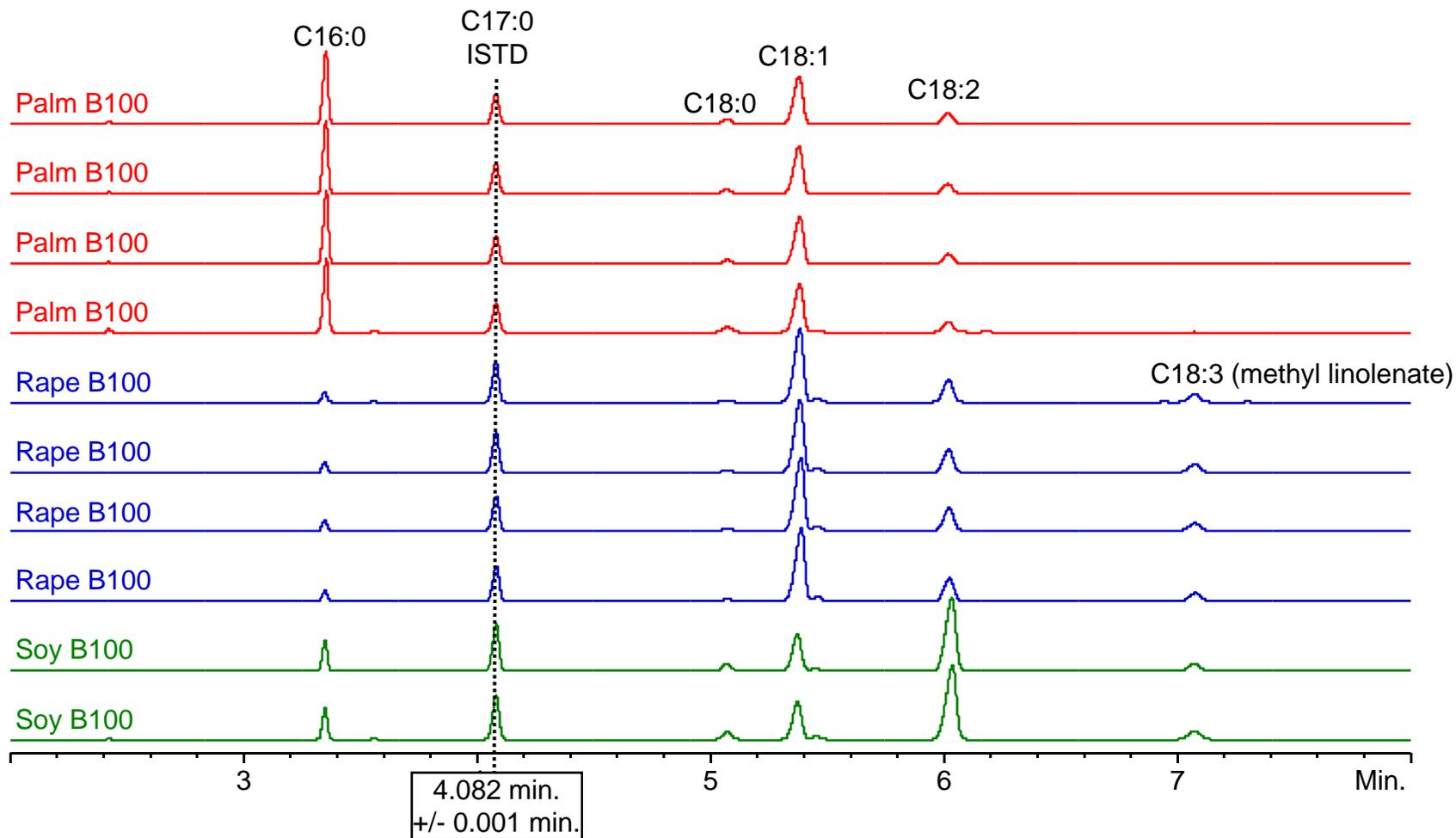
Precise Oven Temperature Control Provides Precise Retention Times
