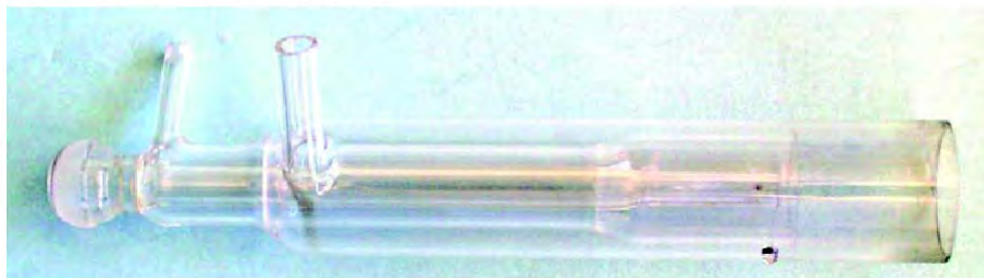
Figure 2. Plasma torch after at least 1,000 hours of use. Clear except for a slight "feather" of brown at the coolant gas entry tube, and a general darkening at the open end of the torch. Argon gas was delivered through the plasticizer-free polyurethane tubing.
