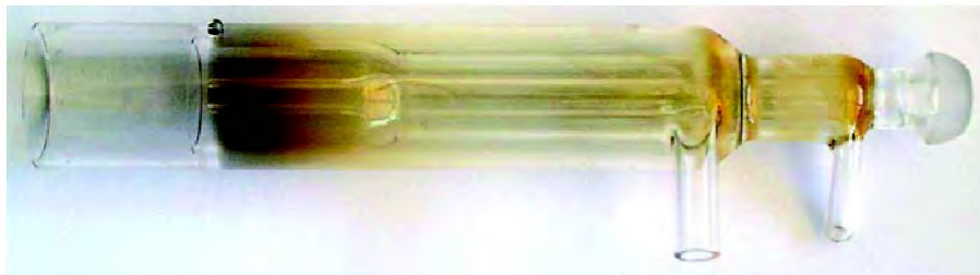
Figure 1. Heavy brown deposit on inside of plasma torch after hundreds of hours use. Argon gas was delivered through the standard plasticized PVC tubing.
