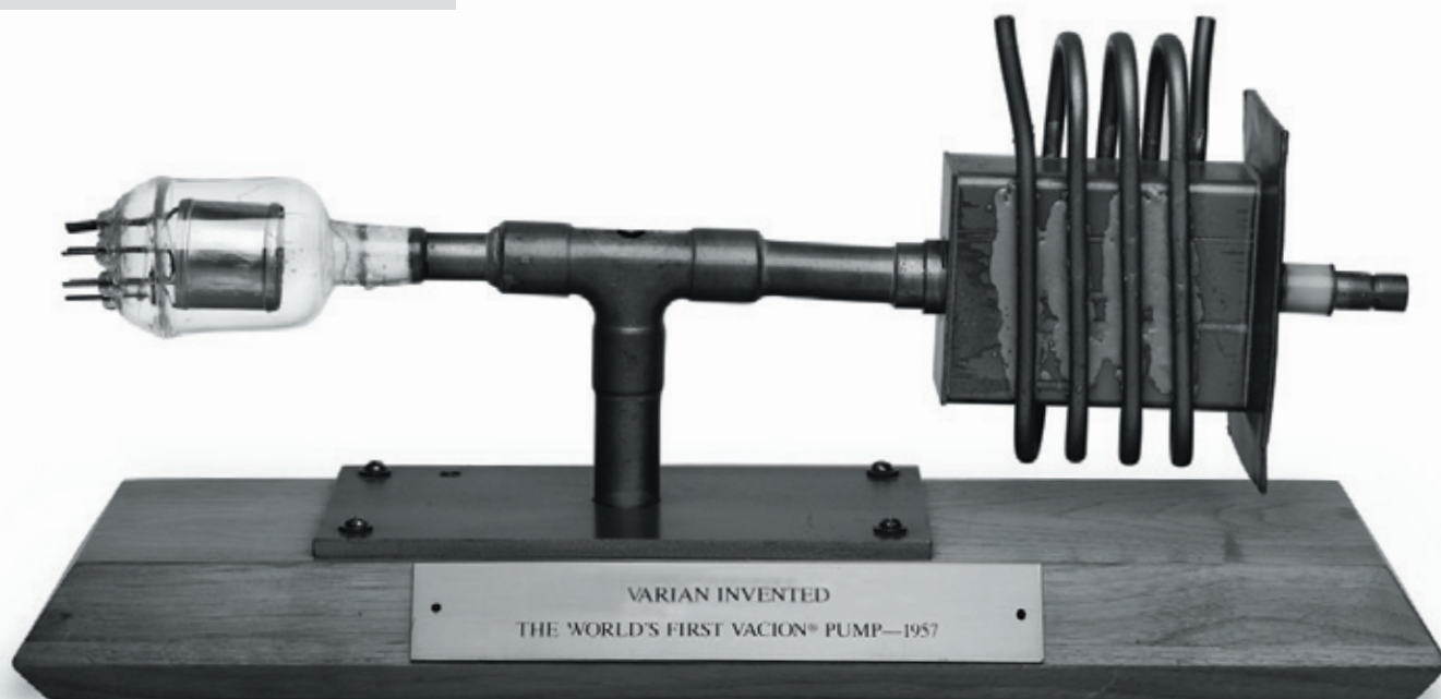
Fig. 1 - The first Vaclon, sputter ion pump was invented by Varian in 1957.
