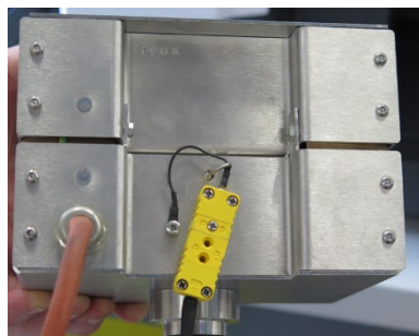
Figure 6. Temperature cable connected to the workhead. An older style cell heater cable is shown.
