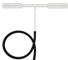
Figure 10. Black fluoroelastomer tubing on the inlet cell stem
