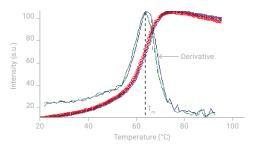
**Figure 5.**  $T_m$  value using 13mer DABCYL labelled PNA probe with 5' 6-carboxyfluorescein labelled DNA.  $T_m$  was calculated by performing a derivative curve using the Cary Eclipse thermal software. It was calculated to be 63.9 °C.
