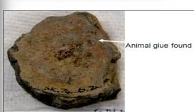
FTIR analysis can determine if tell-tale chemicals are present that indicate recent repair of object and also determine how the object was used.
