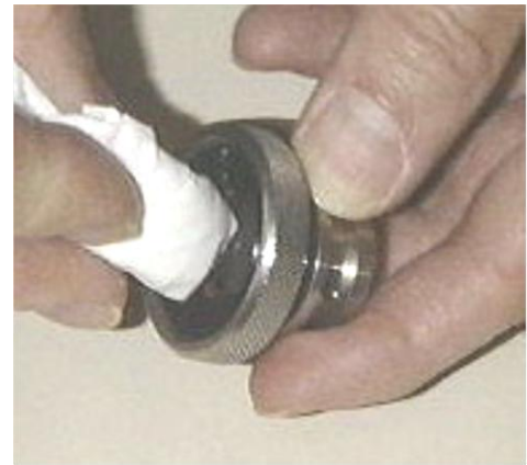
Cleaning end windows from furnace workhead
