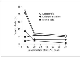
Figure 2. The effect of salt concentration in the mobile phase on peak
