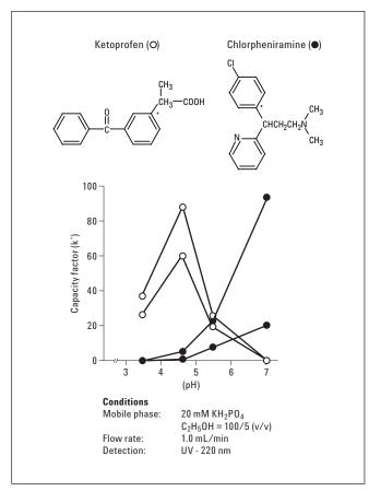
Figure 1. Typical relationship between mobile phase pH and solute capacity factors (k').
