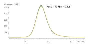
This overlay of 10 chromatograms shows superior retention time precision of the 1290 Infinity II High Speed Pump of 0.005 %RSD, even for ultrafast separations.
