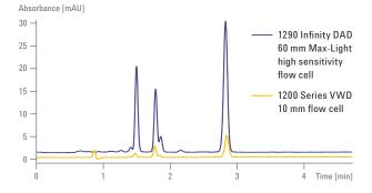
The 1290 Infinity II DAD achieves 10x higher sensitivity than earlier 1200 Series diode array or variable wavelength detectors.
