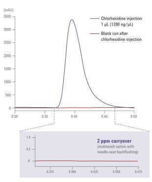
Even with problematic samples the 1290 Infinity II Multisampler can keep carryover down to less than 9 ppm.
