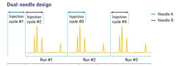
The dual-needle design of the 1290 Infinity II Multisampler eliminates wait times by overlapping injection cycles without compromising data quality by carryover or sample discrimination.
