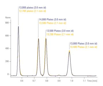
Thanks to lowest extra-column volume the 1290 Infinity II LC achieves highest chromatographic efficiency in terms of plate numbers for both 2.1 mm and larger inside diameter columns.
