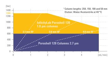
The power range of the 1290 Infinity II LC gives you the flexibility to meet virtually any separation challenge.
