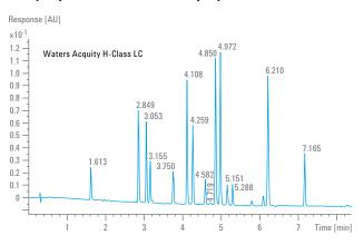
Final separation of the test sample on the Waters Acquity H-Class system using the InfinityLab Poroshell 120 PFP column, applying a gradient from 10 to 47 % acetonitrile over 7.4 minutes, and at a column temperature of 40 °C.
