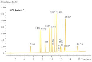
Final separation of the test sample obtained on the target system, the Agilent 1100 Series LC.
