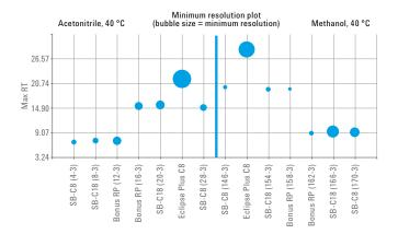
Bubble plots visualize the maximum resolution for separation of complex samples on different columns, enabling a comparison of two different solvent combinations. For details, see Agilent Technical Overview, publication number 5991-6938EN.
