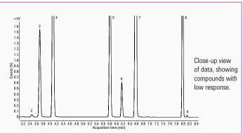
Outstanding repeatability for analyzing residual solvents. For QA labs, the MSD configuration is particularity useful for unknown identification, or for unambiguous confirmation. (SIM/Scan data appear in the table above.)
