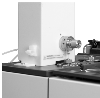
Agilent pneumatic air actuator/valve assembly installed on the 7890A.
