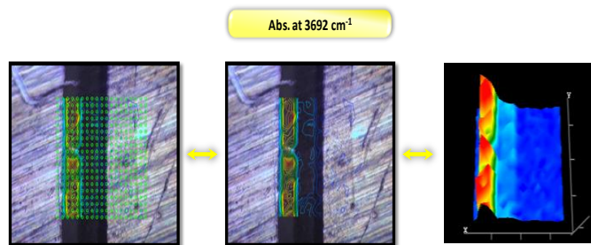
Figure 3. A feature image generated from a spectral peak that is unique to one layer of the paint chip (left), the same feature image shown without the spectral acquisition grid for clarity (center), and the 3-dimensional view of the feature image (right). These images were generated by plotting the intensity of the peak at 3692\text{ cm}^{-1} in the spectrum from each pixel across the entire infrared map.
