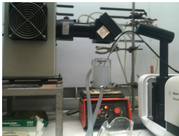
Figure 1. The Cary 60 UV-Vis fitted with the fiber optics microprobe accessory provides a simple mechanism to measure a sample in situ and remote to the instrument
